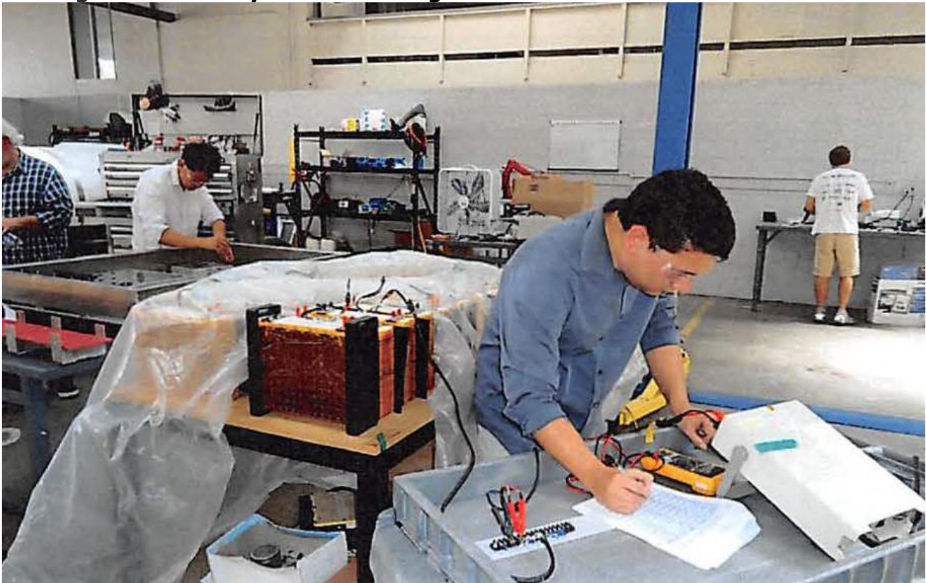
Figure 20: Battery Module Testing Prior to Installation into RailScout EV
