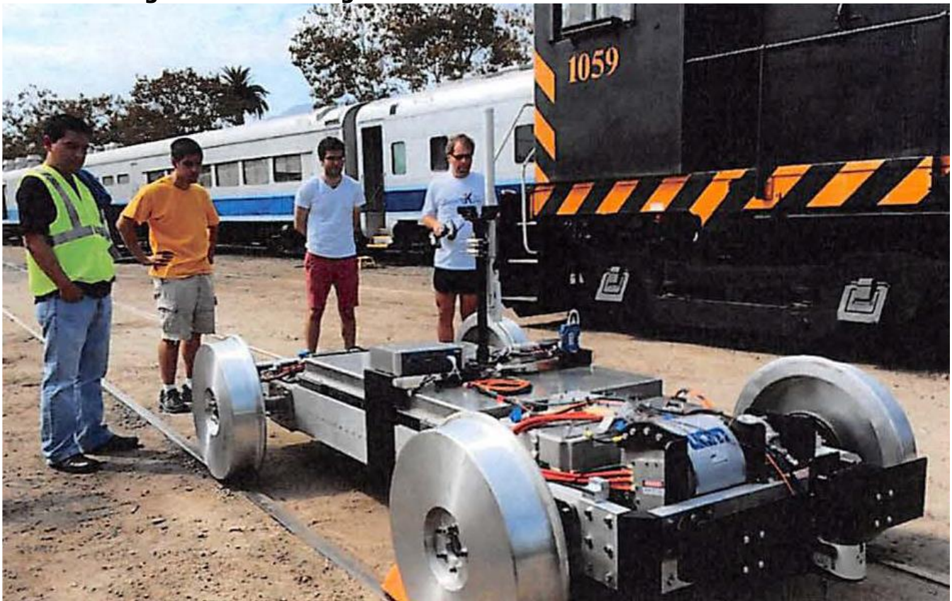
Figure 30: Powering on the RailScout at the Fillmore Test Site
