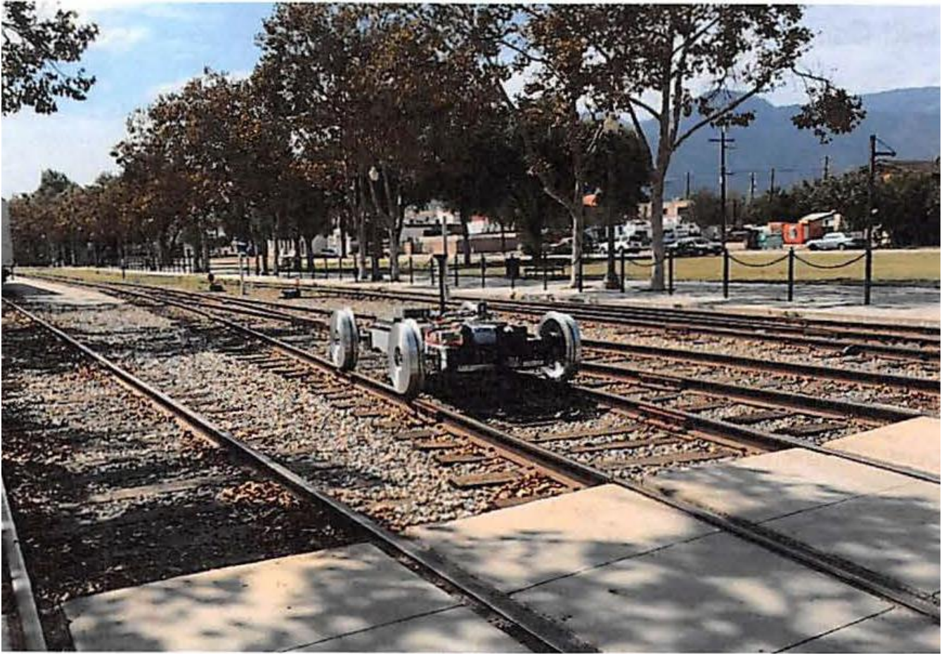
Figure 35: RailScout in Full Automated Operation
