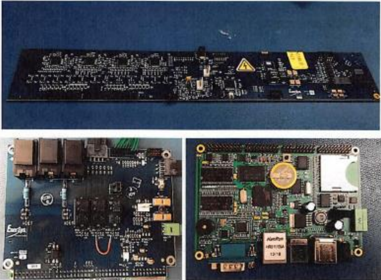
Figure 10: Control Board (top), Interface Board ( bottom left) and Single Board Computer (bottom right)
