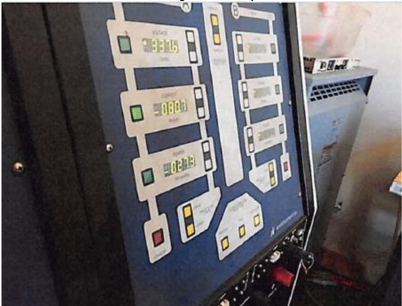
Figure 27: Display of High Voltage Charger Showing Battery at 337.6 Volts being discharged at -80.7Amps
