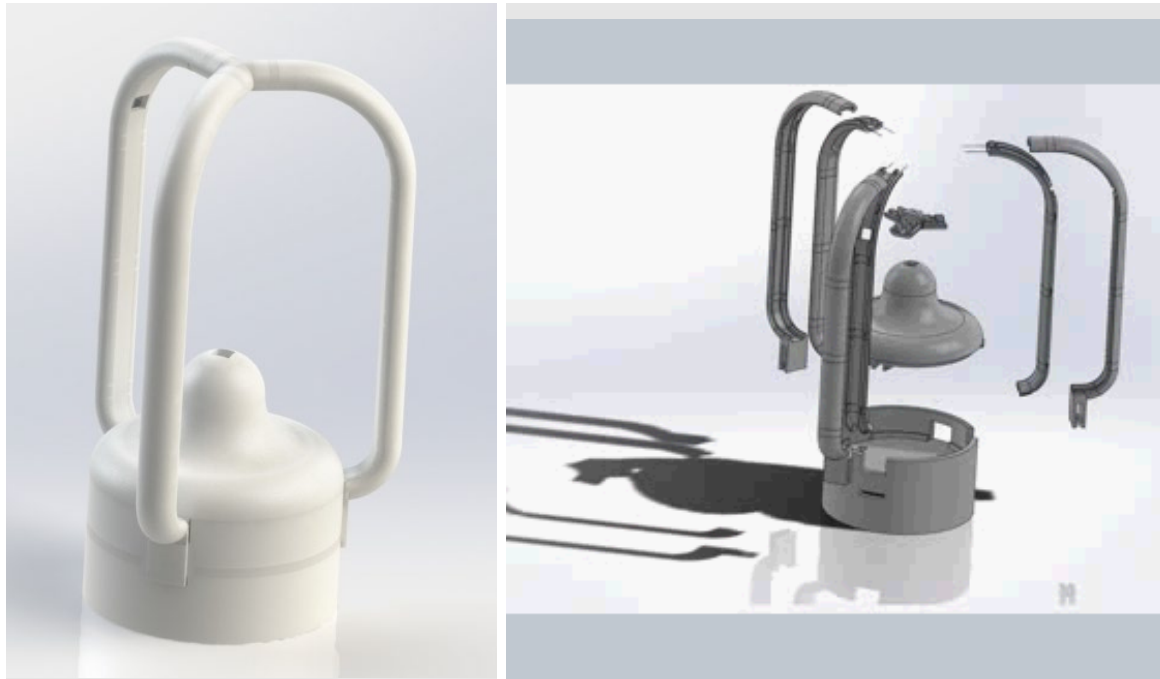
Left: the 3-D printed support system for the first room anemometer prototype, with sensors embedded in the vertical support arms. Right: an exploded view SolidWorks rendering of support system.
