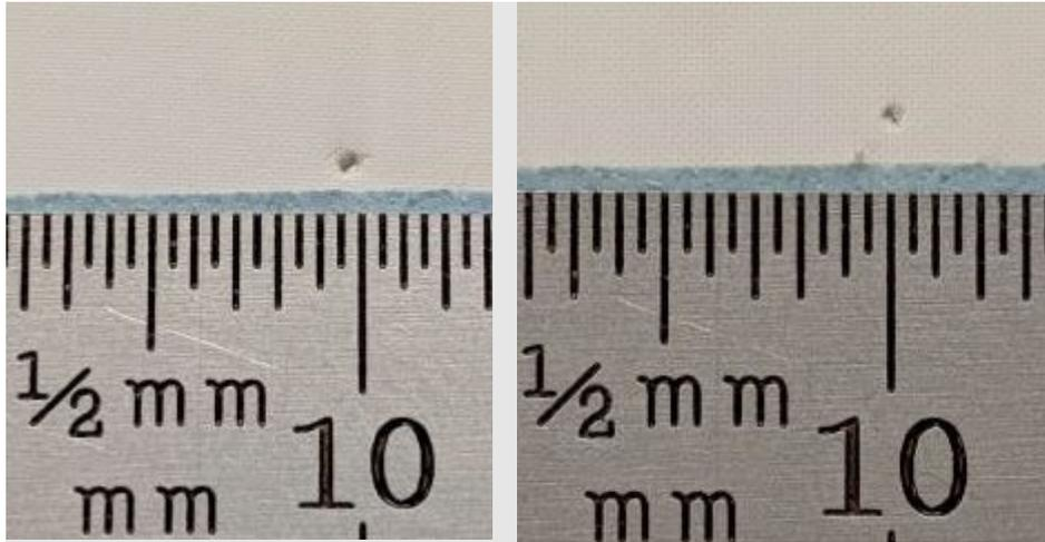
**Two of the four pinholes created within a PFO-100 FO membrane element with 33 sheets total.**
