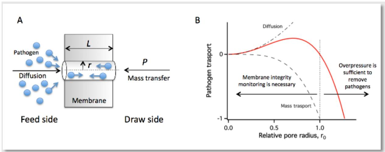
**(A) Schematic of constituent (such as, pathogens or molecules) diffusion through a cylindrical pore retarded by overpressure "P."**
