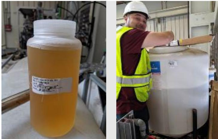
**MS2 concentrate (left) spiked into a feed tank (right) of RO concentrate for the MS2 spike test.**
