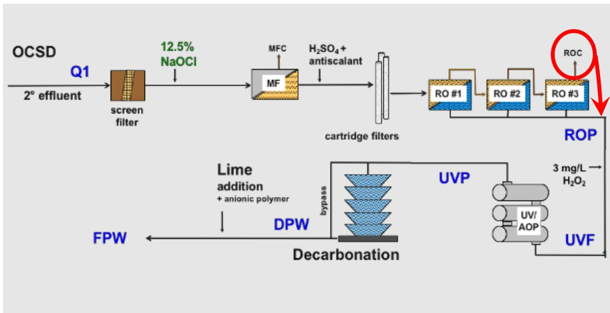
**A red circle and arrow indicating the DPRShield pilot treated water in the reverse osmosis concentrate brine waste stream with the goal of producing water similar to the ROP (RO permeate) stream.**
