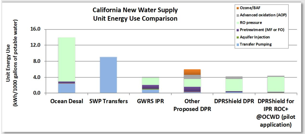
**Energy use comparison for production of potable water from different water sources available in California. State log removal credits required for permitting are assumed for each process.**
