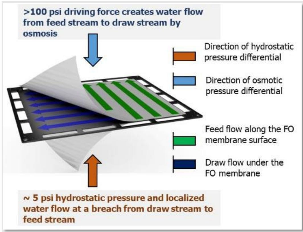
**Alternate Breach-Activated Barrier illustration on single membrane plate within a PFO-100 element.**
