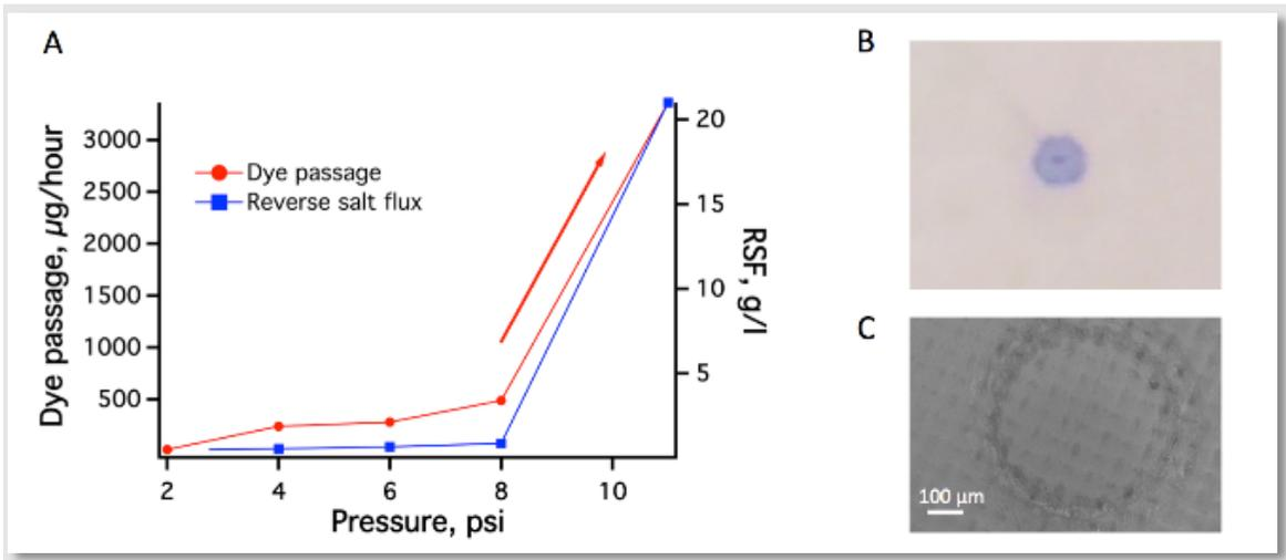
**(A)** Dye passage and RSF as a function of differential pressure between the draw and feed side of an FO membrane damaged by a sharp spacer. **(B)** Optical image of a damaged area stained with methylene blue, and **(C)** scanning electron microscopy of the same area.
