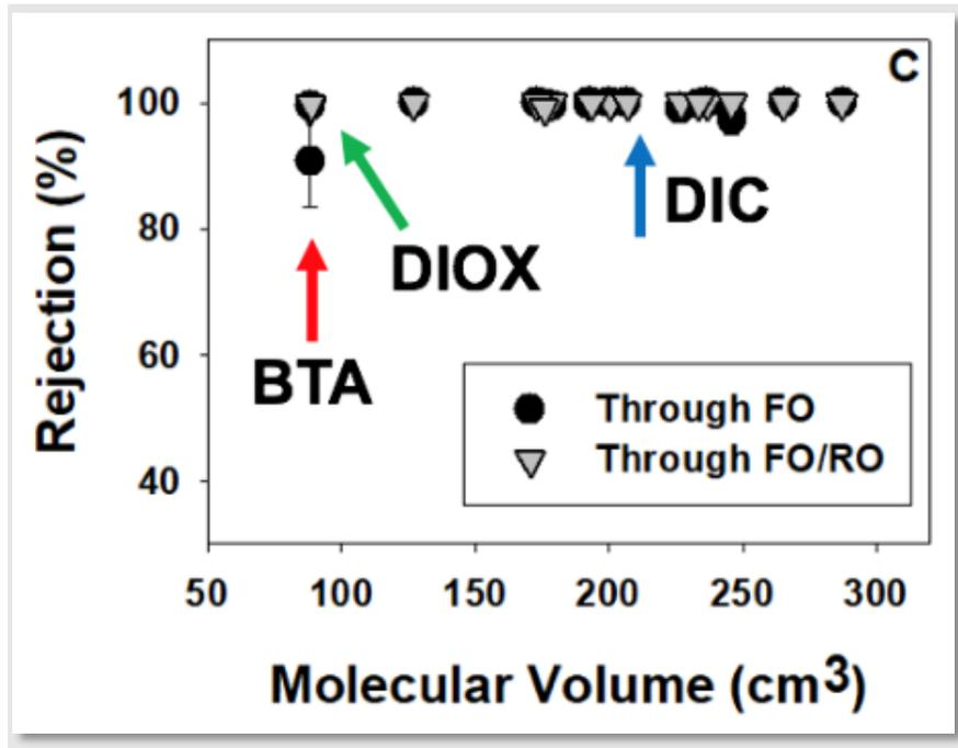
Percent rejection of 15 organic contaminants by the FO membrane alone (comparing the concentrations in the FO influent and draw solution) and by the combined FO/RO system (comparing the FO influent and RO effluent concentrations) for treatment of RO concentrate. Error bars represent the standard deviation of three sampling events. BTA= benzotriazole, DIOX = 1,4-dioxane, DIC=diclofenac.
