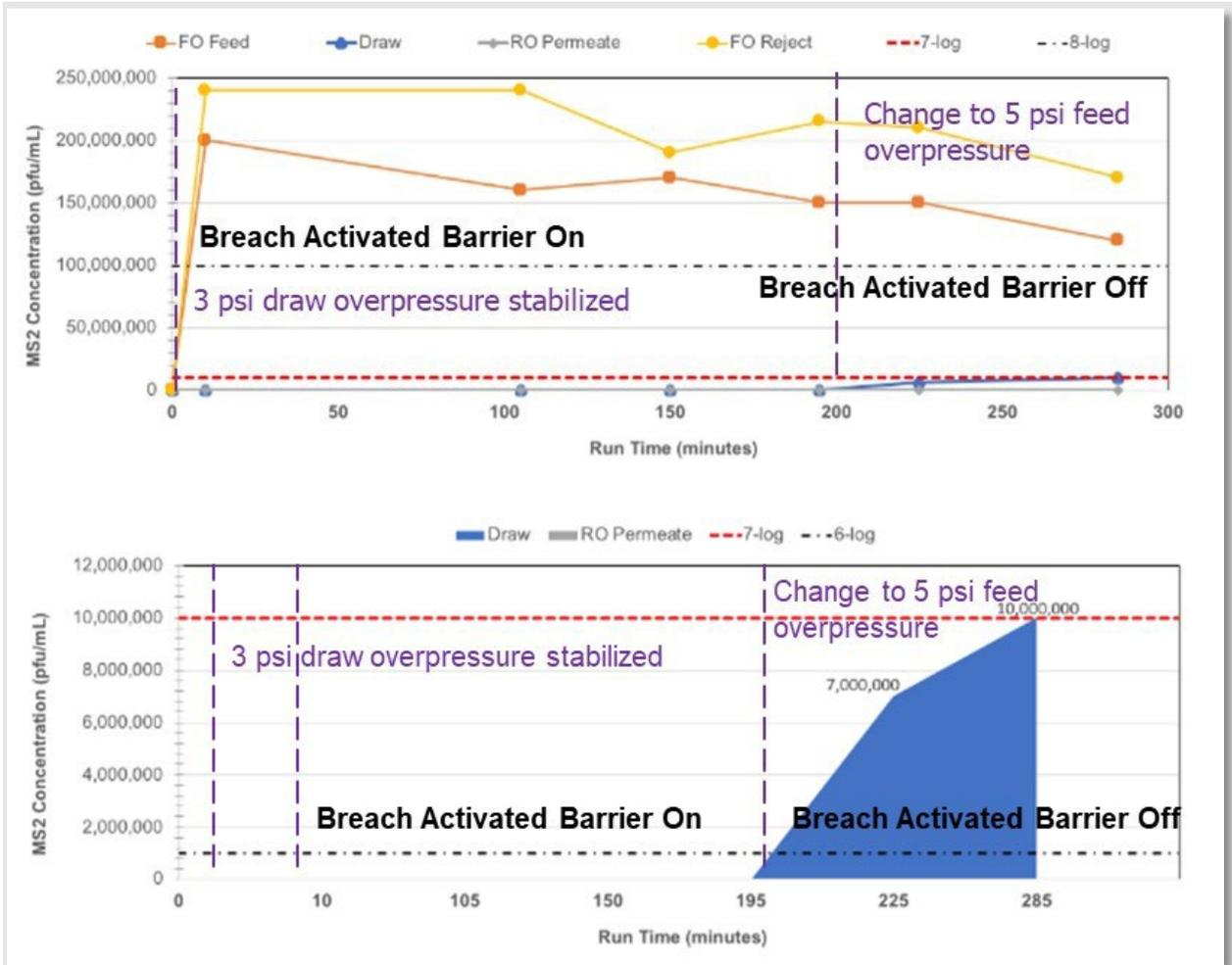
**MS2 spiking data in all process stream (Top) and FO draw and RO permeate data only (Bottom).**
