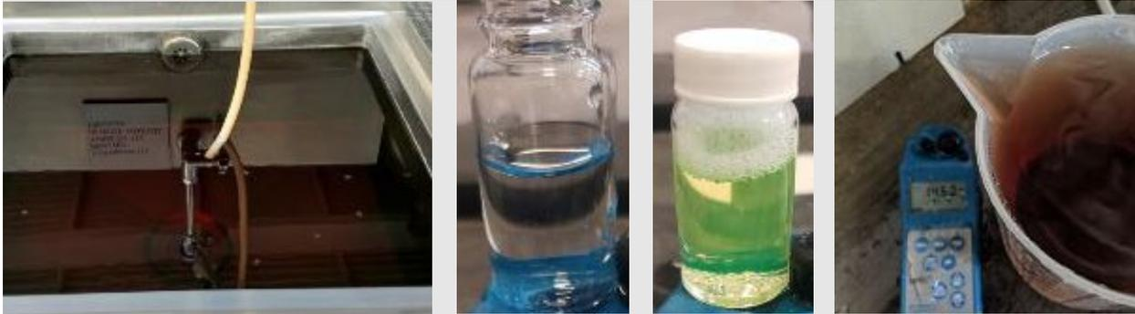
**DPRShield feed water (left), permeate (center left), draw with dye (center right) and FO reject (right).**
