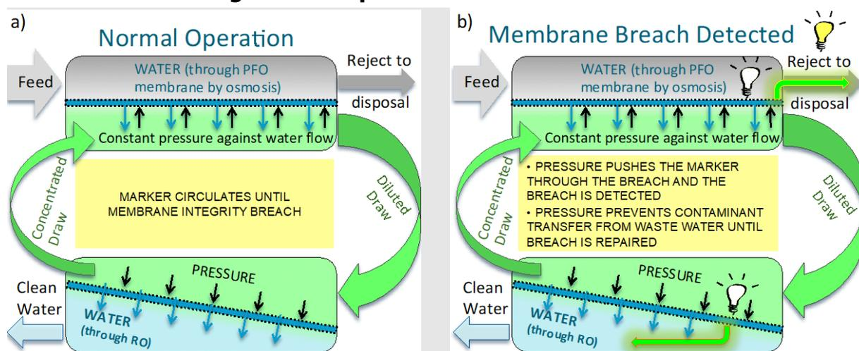
**Schematic of DPRShield System with Breach-Activated Barrier technology under normal operation (a) and when breach is detected (b).**
