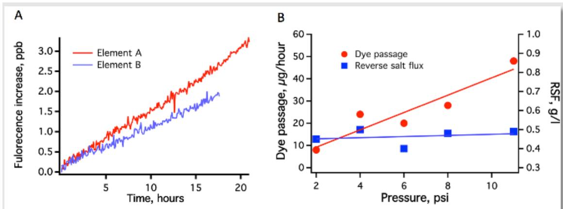
**Fluorescence increase due to dye passage through a Porifera PFO-20 element with 2 psidraw overpressure and (B) dye passage and RSF as a function of draw overpressure.**
