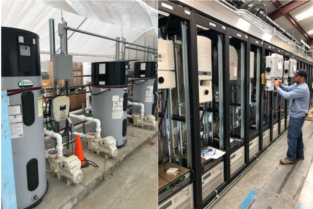
Figure 9: Smart Loads and Smart Inverter Test Setup at PG&E Laboratory
