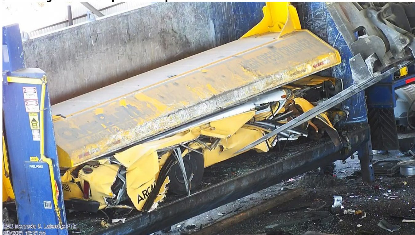
Figure 2: Example of Acceptable Method to Dismantle Vehicle Chassis
