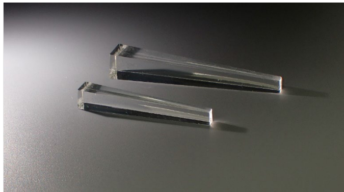
Figure 34: Experimental Couplers of the Newly Developed Designs Made Using Injection Molding
