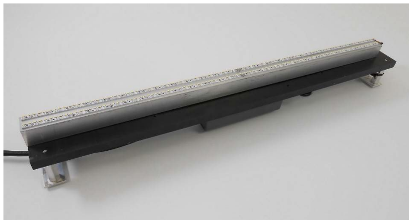
Figure 13: Test LED Module Assembly
