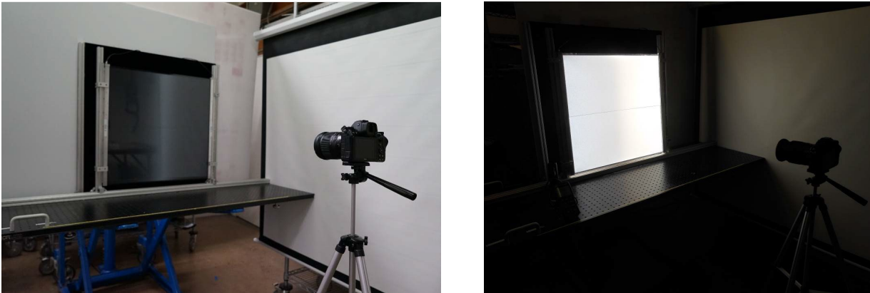
Figure 27: Test Bench for Assessing Uniformity of Lighting Panel Prototypes (left) and HDRI Measurements of the LED-illuminated Panel (right)
