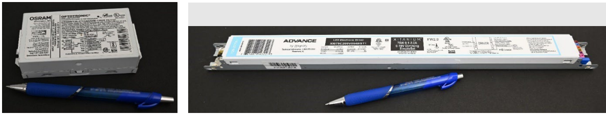
Figure 38: LED Drivers Selected for Final Prototyping and Lighting System Integration
