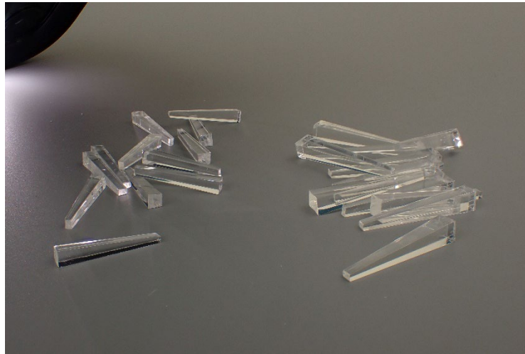
Figure 35: Optical Couplers Made Using the Full-production Run
