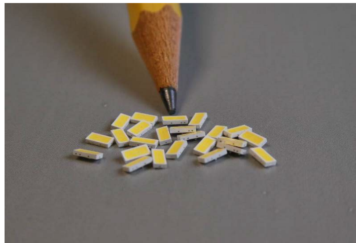
Figure 9: Mid-power LED Packages Used for Making New Linear LED Modules
