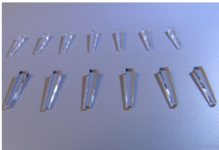
Figure 30: Selection of Experimental Optical Couplers Produced With Different Surface Finishes
