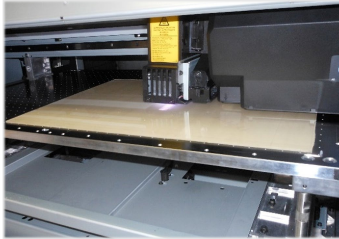
Figure 21: Substrate Patterning Using UV Microprinting Process
