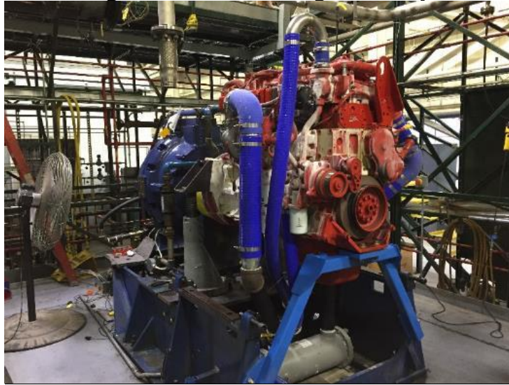
Figure 3: ISX12N Engine Setup
