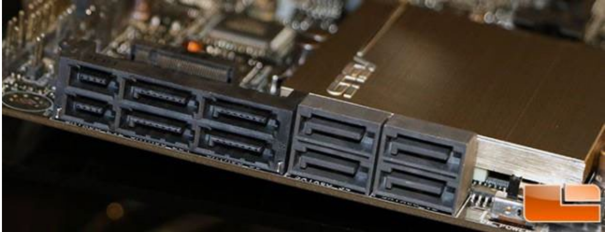
Figure 2. SATA connectors with SATA or SATA Express (Image source: Legitreviews.com)
