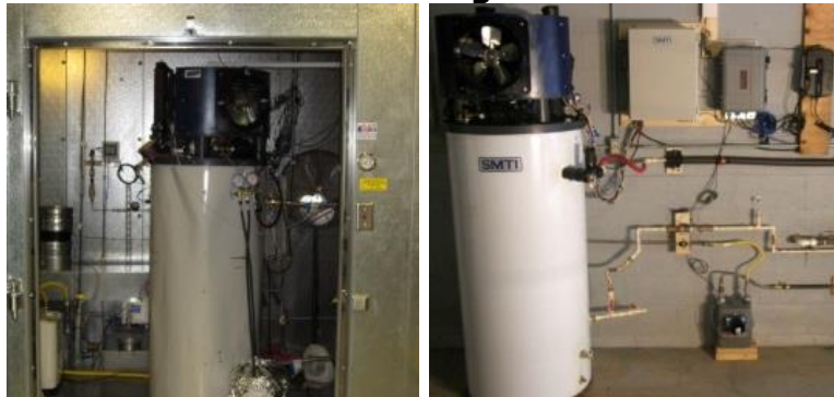
Figure 22: Early Gas Heat Pump Water Heater Prototypes in GTI Lab and Field Testing
