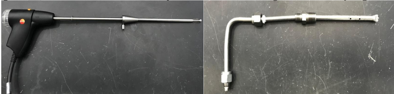
Figure 29: Testo Portable Gas Analyzer and Custom Integrated 4" Sampling Probe
