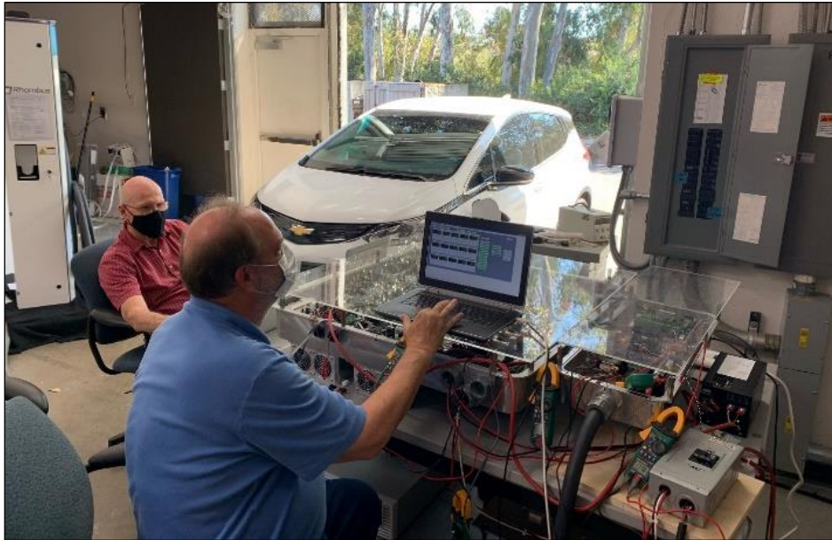
Figure 10: Testing SPIN System Charging and Discharging with a Chevy Bolt
