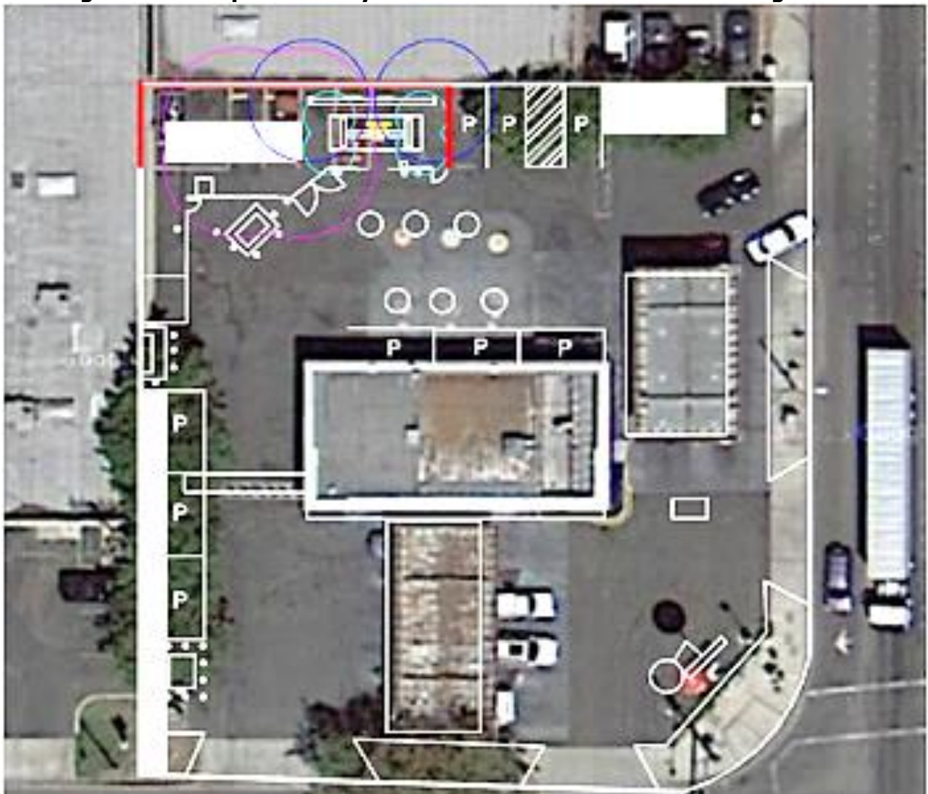
Figure 2: Air Liquide site layout at the Anaheim California fueling station
