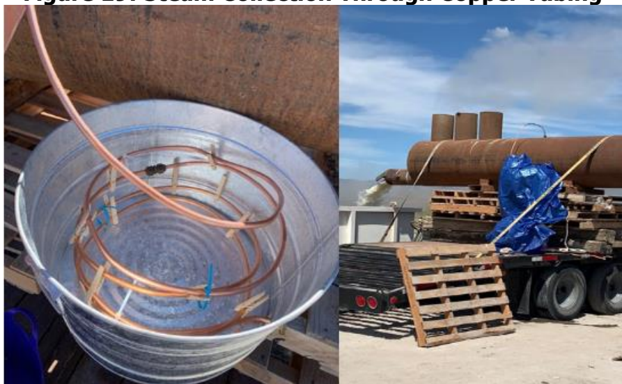
Left: Copper tubing plumbed into flash chamber. Right: Blue tarp covering bucket with copper tubing filled with ice and plumbed into flash chamber.
