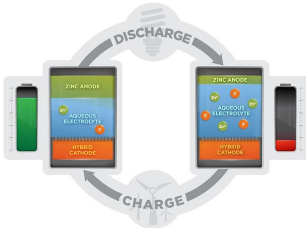
Figure 9: Simplified Schematic of Eos Zinc Hybrid Cathode (Znyth) Technology Zinc Halide Redox
