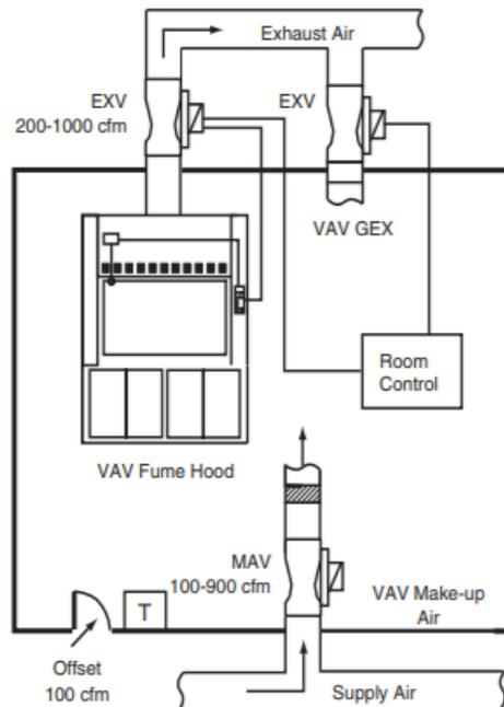
An image of a schematic drawing of Variable Volume Laboratory.
