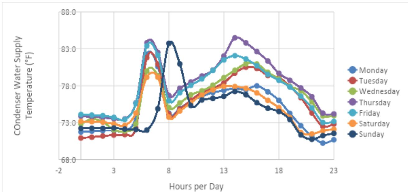
Image of a plot graph that shows the Chiller 1 Average Hourly Condenser Water Supply Temperature by Day.
