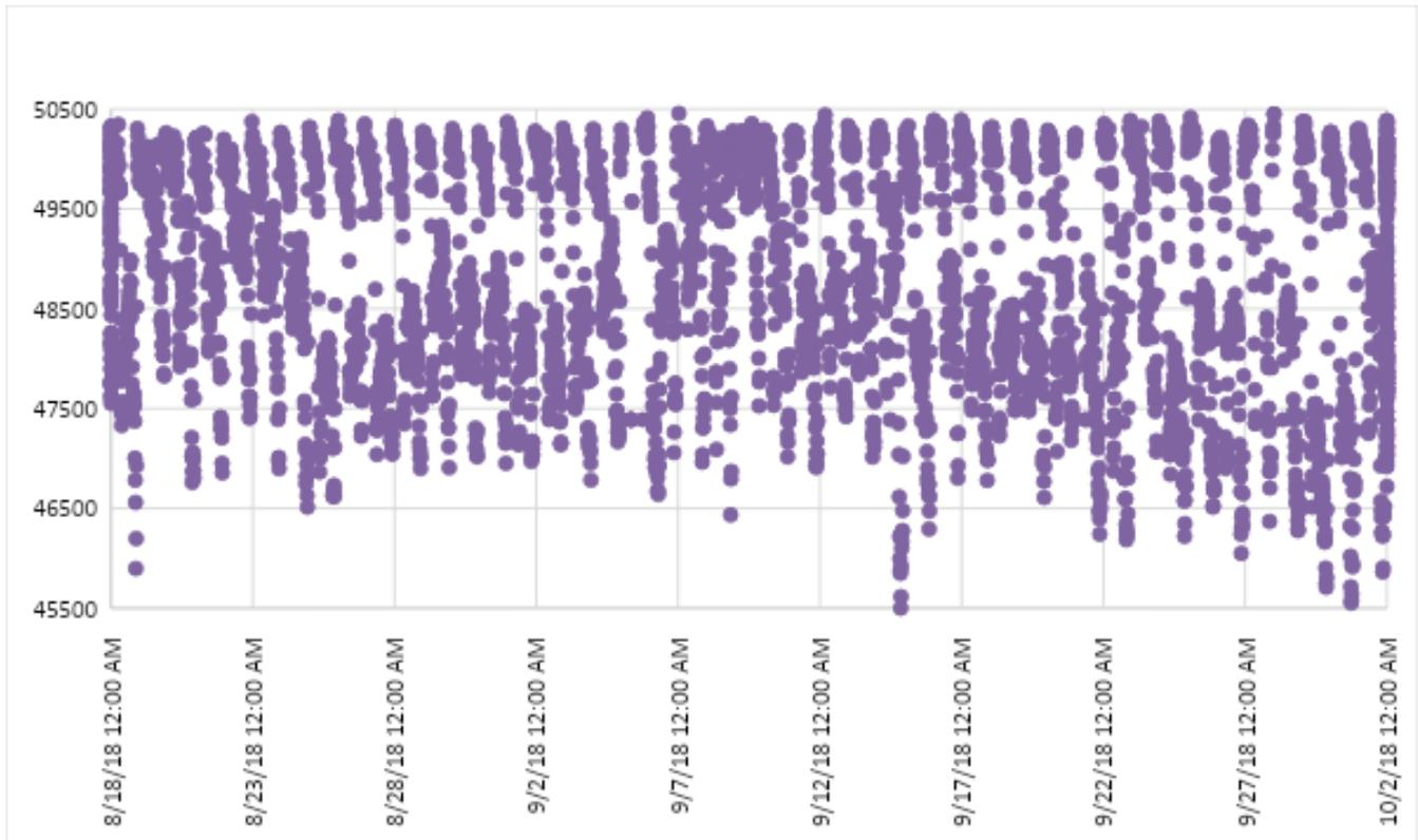
Image of a plot graph that shows the total airflow volume in baseline M&V data from August 18, 2018, to October 2, 2018, of AHU-2.
