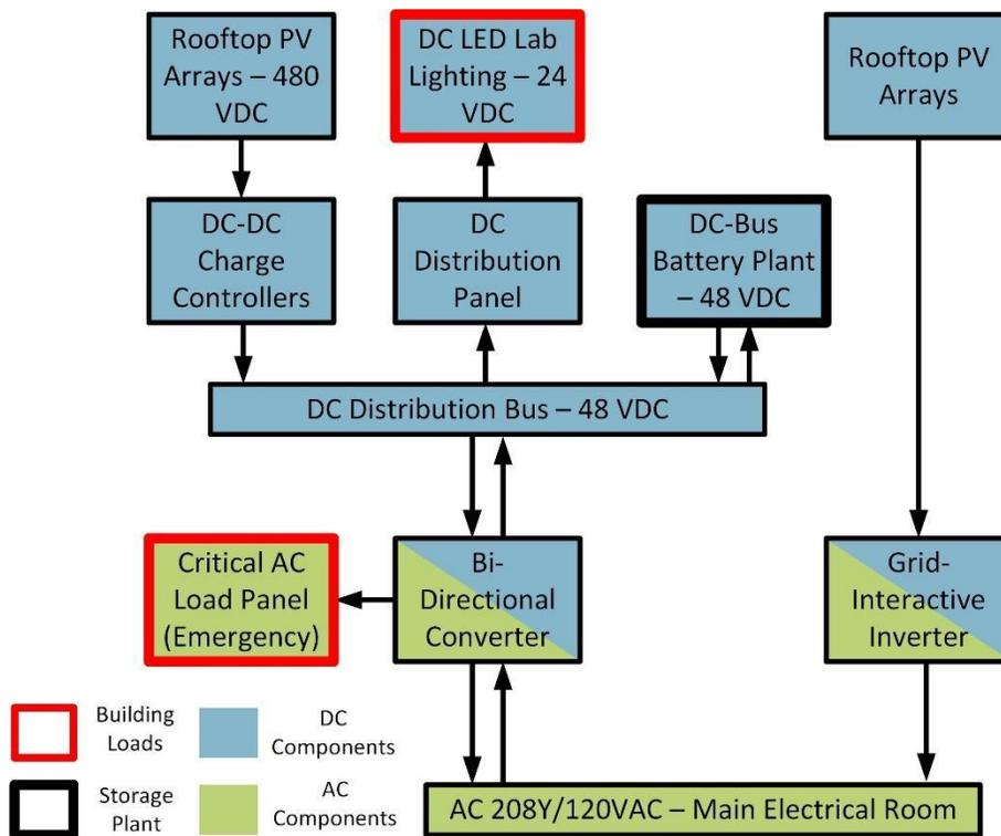
Schematic diagram of the DC lighting system.
