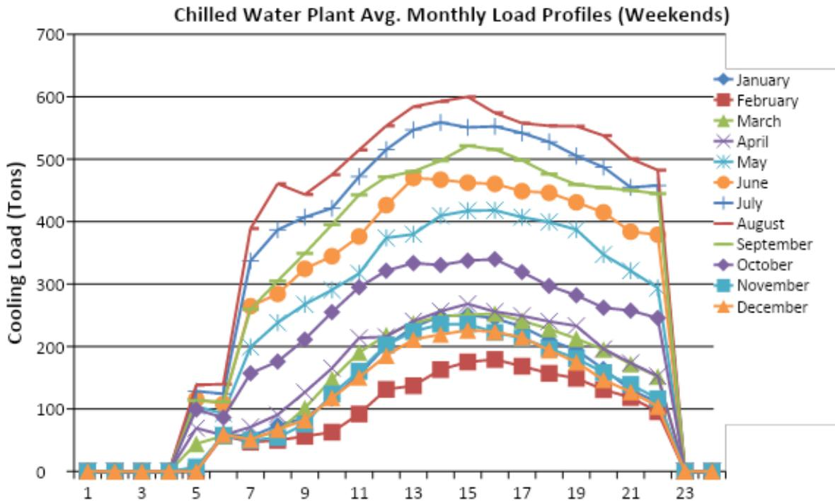
This image is of a plot representing a data set of the chilled water plant cooling load average on monthly load profiles of weekends.
