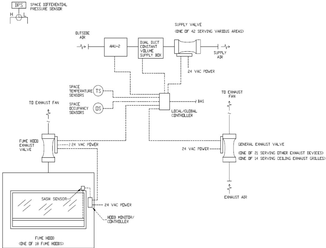
Drawing of Control Valve and Fume Hood Integration.
