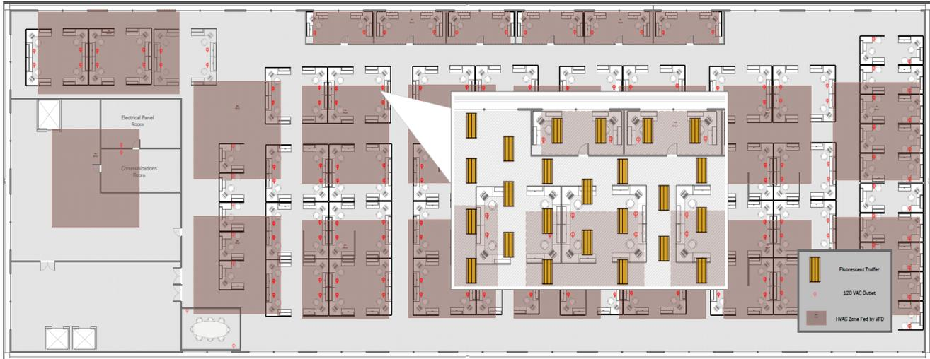
Overhead layout of the office space showing cubicles, overhead lighting, and areas of influence of HVAC.
