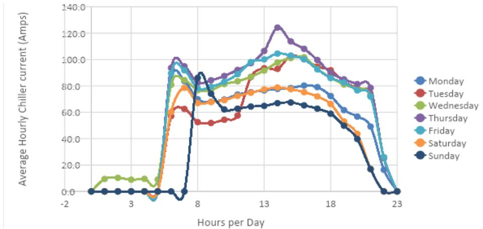
Image of a plot graph for the Operation Profile for Chiller 1 and Chiller 2, combined by Day.
