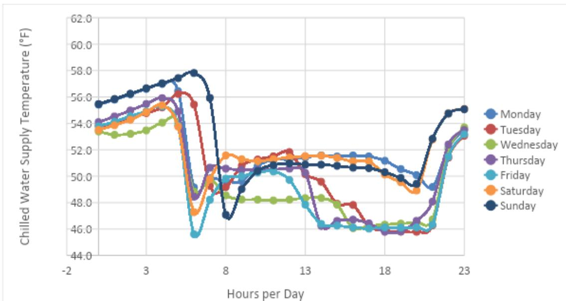
Image of a plot graph that shows the Chiller 1 average Hourly Chilled Water Supply Temperature by Day.
