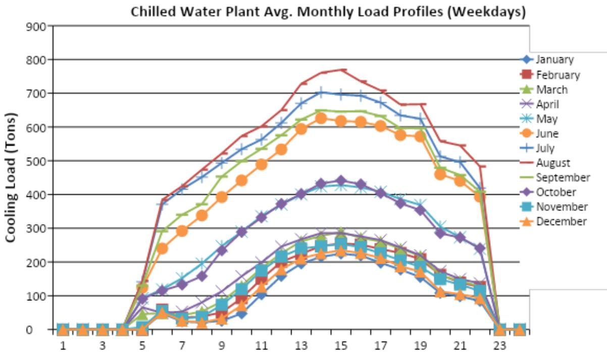
This image is of a plot representing a data set of the chilled water plant cooling load average on monthly load profiles of weekdays.
