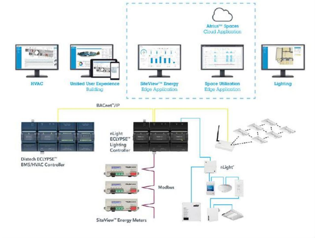
A diagram showing the controls architecture of the nLight lighting system.
