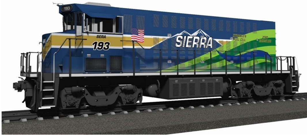
Figure 5: Sierra Northern’s Zero-Emission Hydrogen Switching Locomotive
