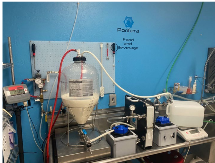
Figure 26: FO Concentration of Whole Milk
