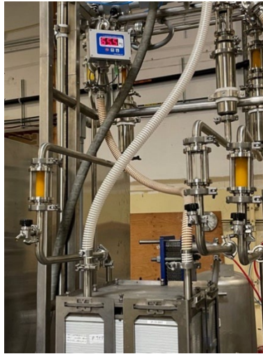
Figure 35: In-Line Refractometer Measuring Orange Juice °Brix
