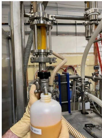
A Porifera team member is collecting OJ concentrate from the third stage of the RC3 system
