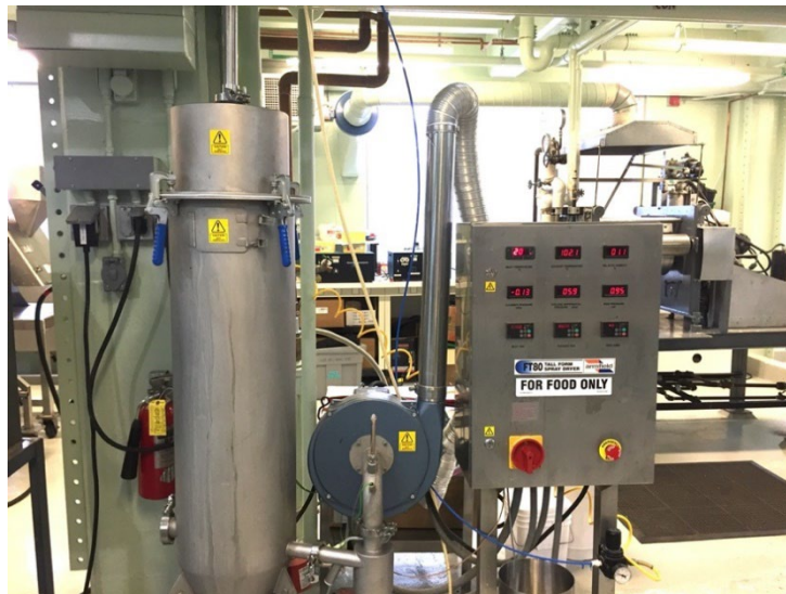
Figure A-6: Pilot Scale Spray Drier at the USDA, Albany, California
