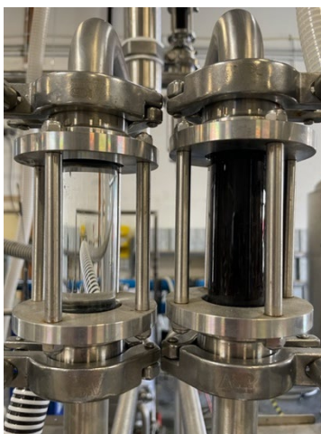
Figure 41: Feed and Draw Lines: Coffee (Right) and Glycerol Solution (Left)
