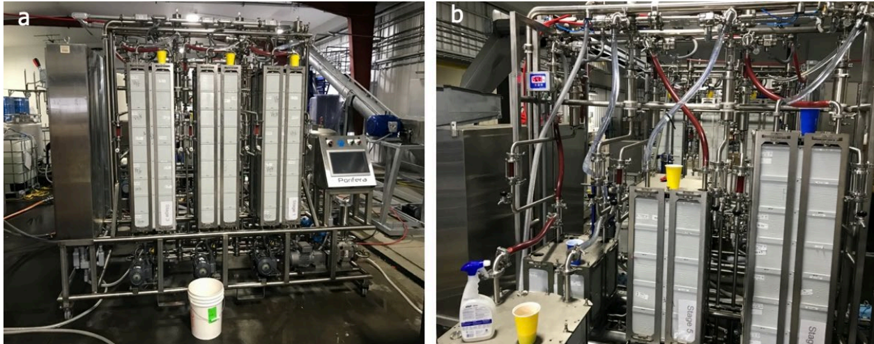
Pictures showing RC6 system concentrating watermelon juice
