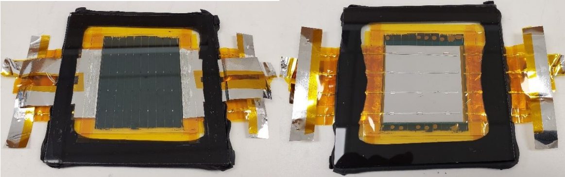
Figure 11. (Left) Perovskite+silicon tandem module viewed from the top, perovskite-facing. (Right) Perovskite+silicon tandem module viewed from the back, silicon-facing.
