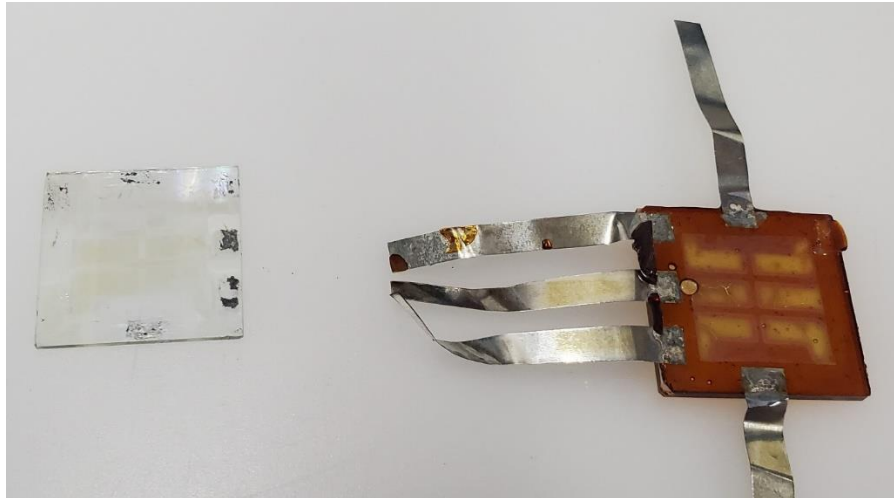
Figure 10. Tandem solar cell subjected to a damp heat test, which completely separated during testing. Lifting the device was enough to separate the two pieces of glass. The actual device is on the left, while the cover glass with epoxy is on the right.
