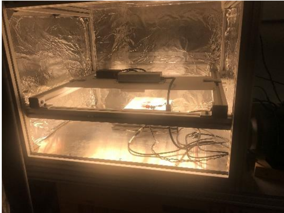
Figure 8. (Top) Custom-Built Constant-Illumination Durability Chamber. Bottom: Operational Curve of a Perovskite Solar Cell Over Thousands of Hours of Continuous Operation
