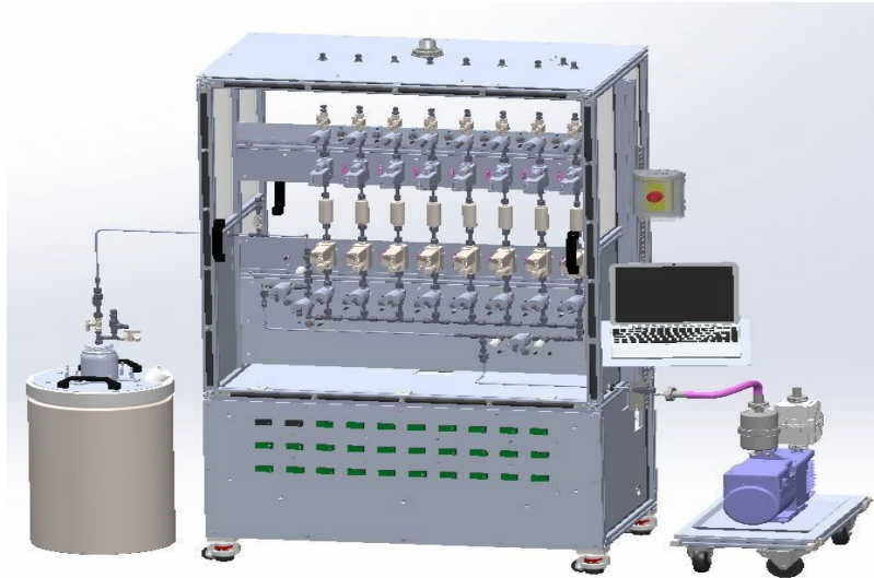
Figure 8: Drawing of Manifold in Enclosure with Electrolyte keg. Drawing of the Final Gas Manifold Design including the Operator Computer, Vacuum Pump, and Electrolyte keg Installed in a Cooling Dewar.
