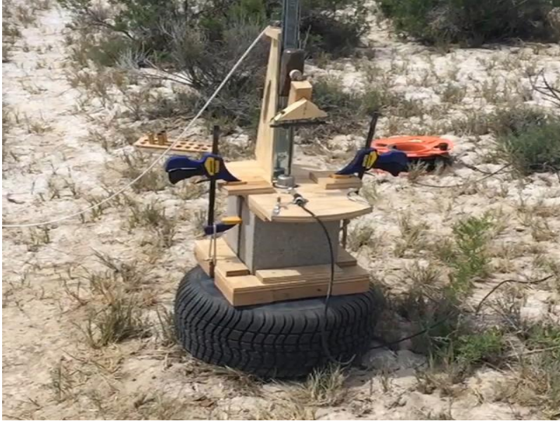
Figure 14: "Betsy Gun" apparatus used as a source for the seismic array.
