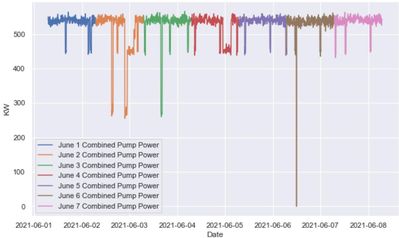
**Graph showing the Cal Water’s Tubeway Station total pump power for the first week of June 2021 in five-minute resolution**
