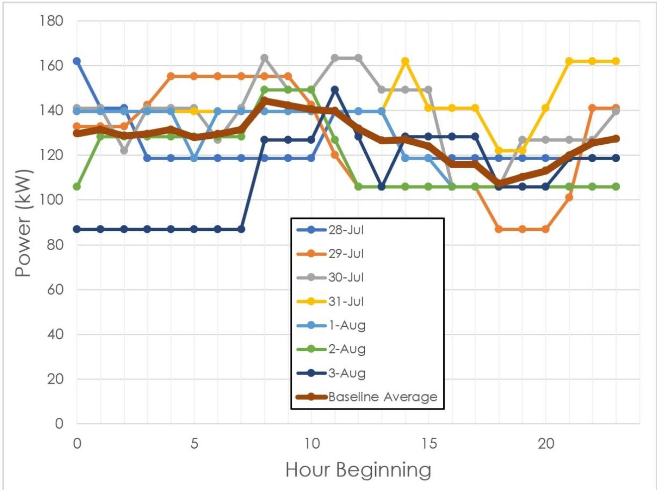
Diagram showing the floor heater baseline developed using seven days of historical data.
