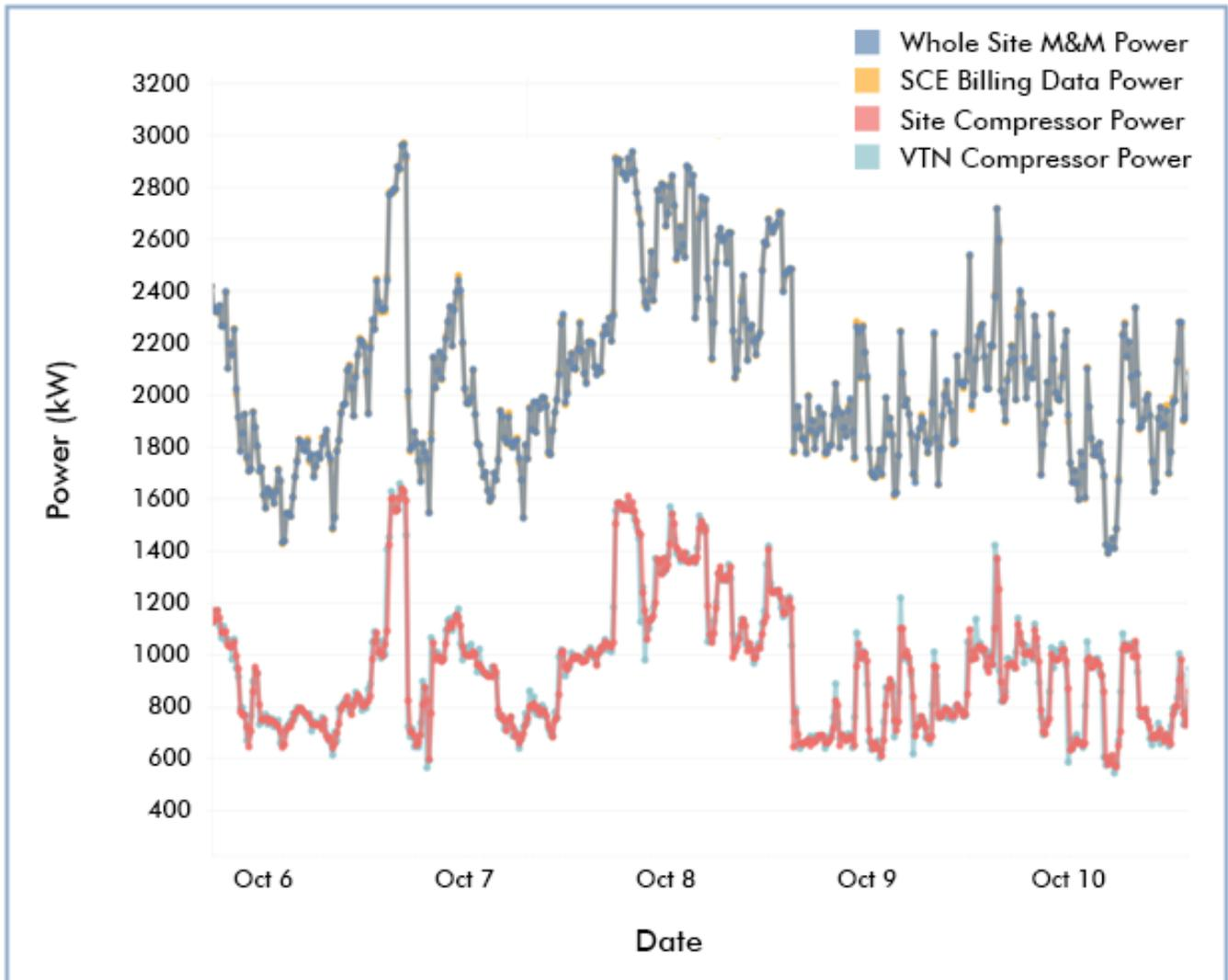
Diagram showing the comparison of various data sources for power metering
