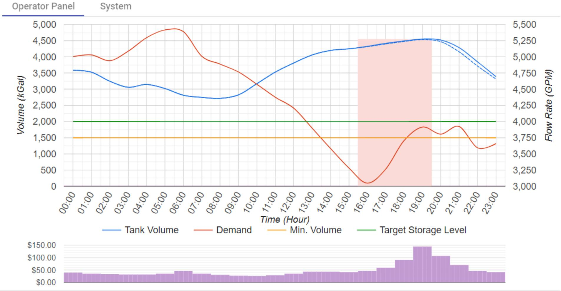
The day-ahead decision support tool displays a graphical representation of forecasted tank volume, demand, minimum volume, and target storage level as they change through the day.
