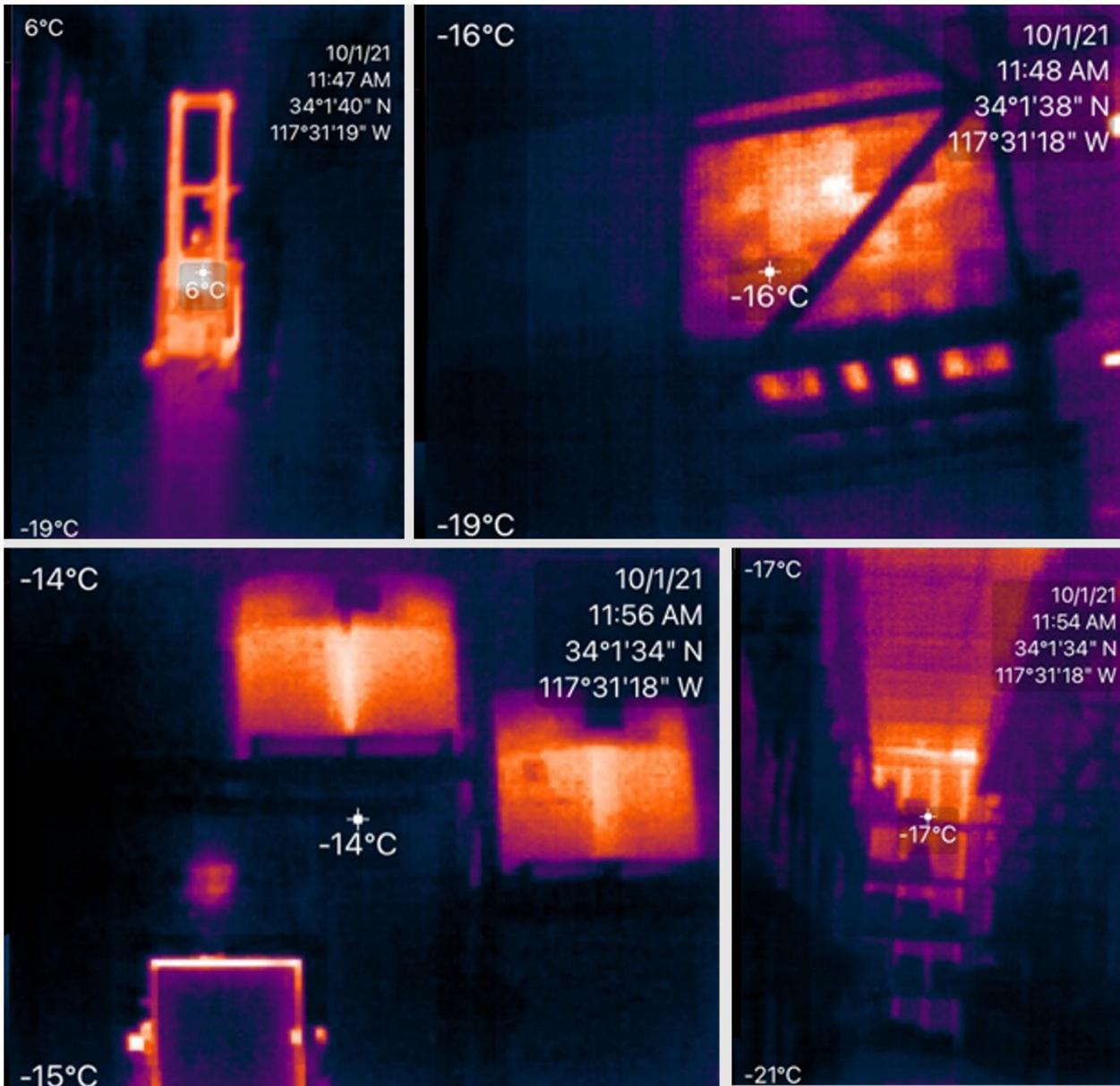
**Sources of heat inside a frozen room (clockwise from top left): an electric forklift, food pallets, food pallets and drums, and perimeter walls and ceiling**
