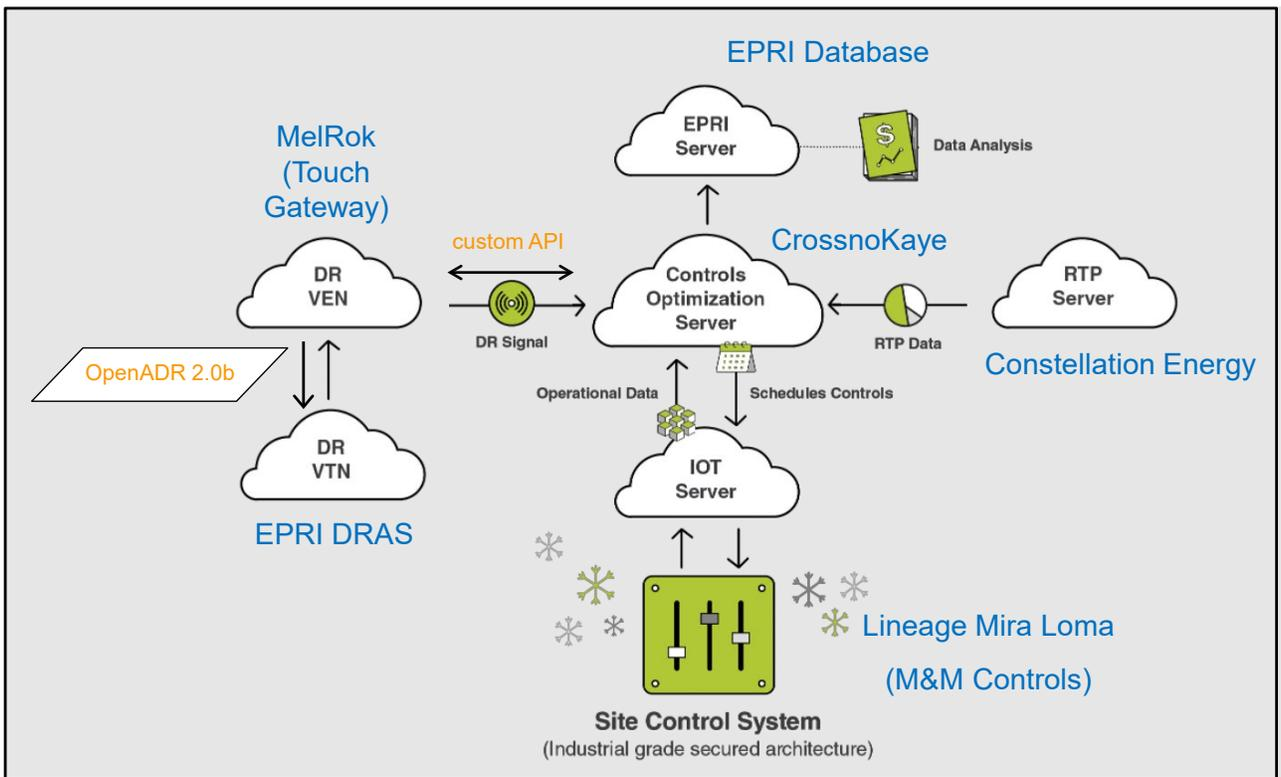
**Diagram for implementing OpenADR 2.0b on the Lineage refrigeration plant with process optimization**
