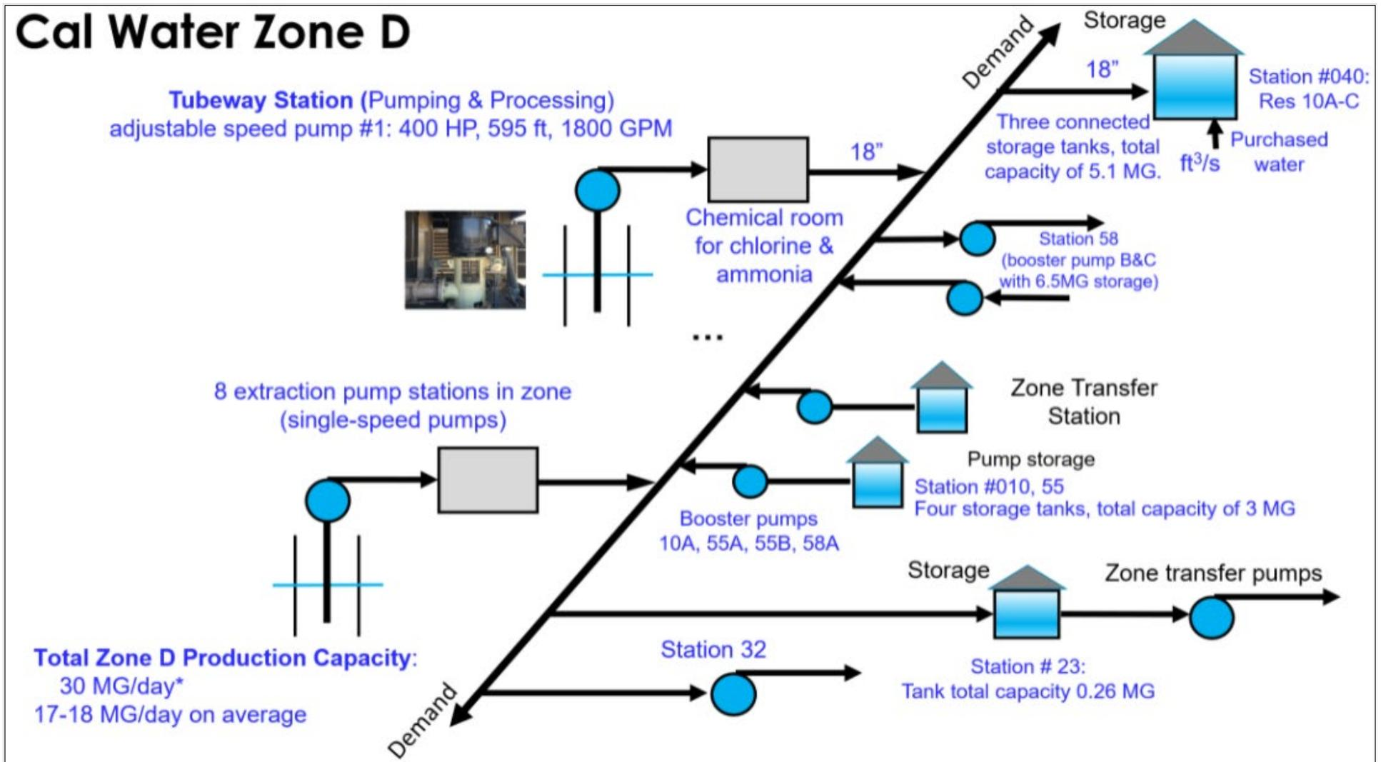
Diagram showing Cal Water zone D system
