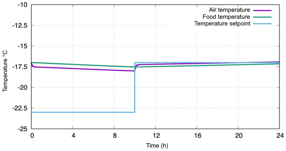
Graph showing the temperatures of a modelled frozen room during a DR temperature setpoint reset.
