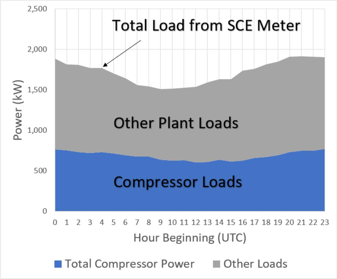
Typical hourly load fluctuation at the Lineage industrial refrigeration site
