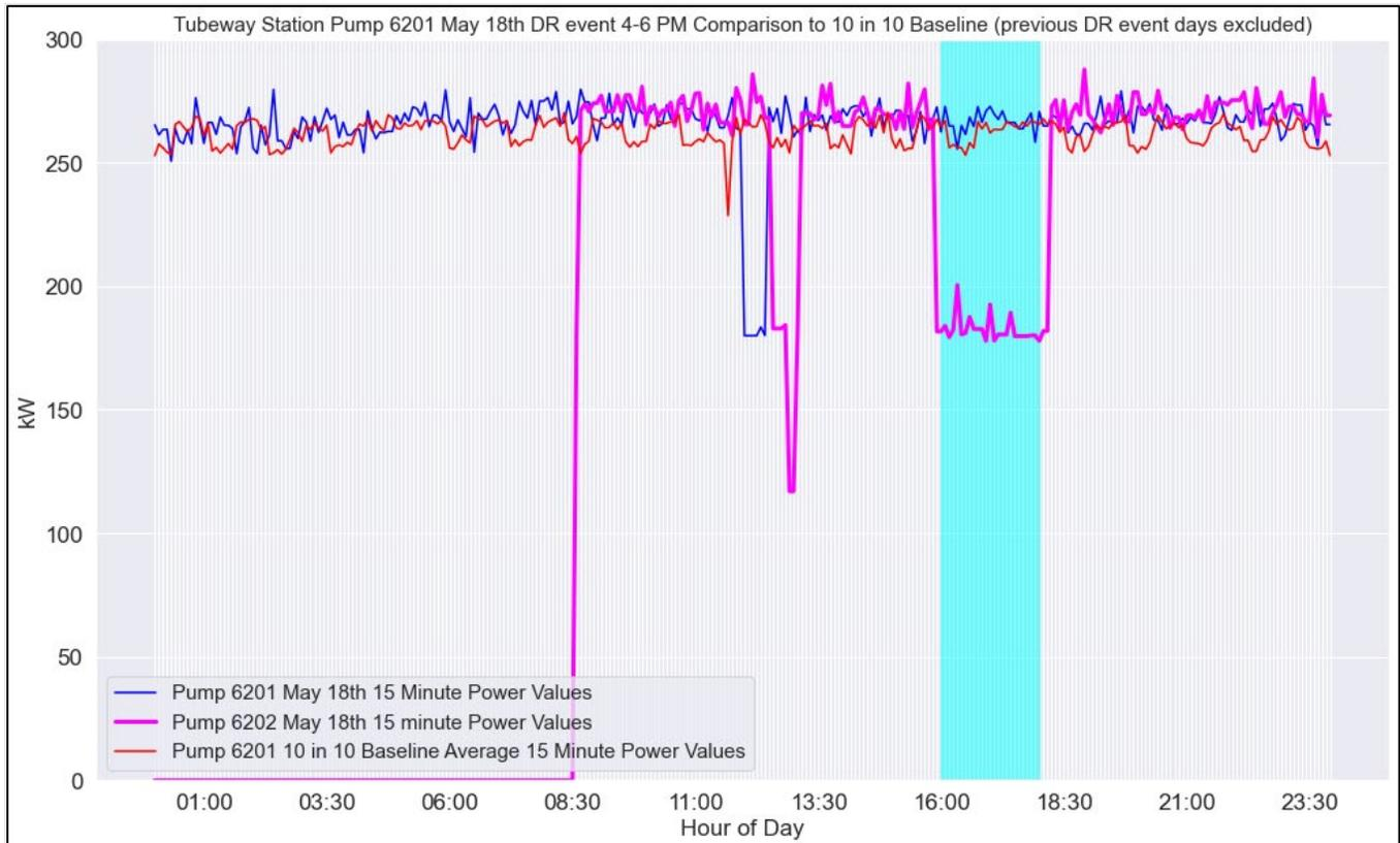
The graph shows an 80-kW reduction from pump 6202 during the May 18, 2021, DR event from 4:00 p.m. to 6:00 p.m. compared to the pump 6201 10-in-10 baseline
