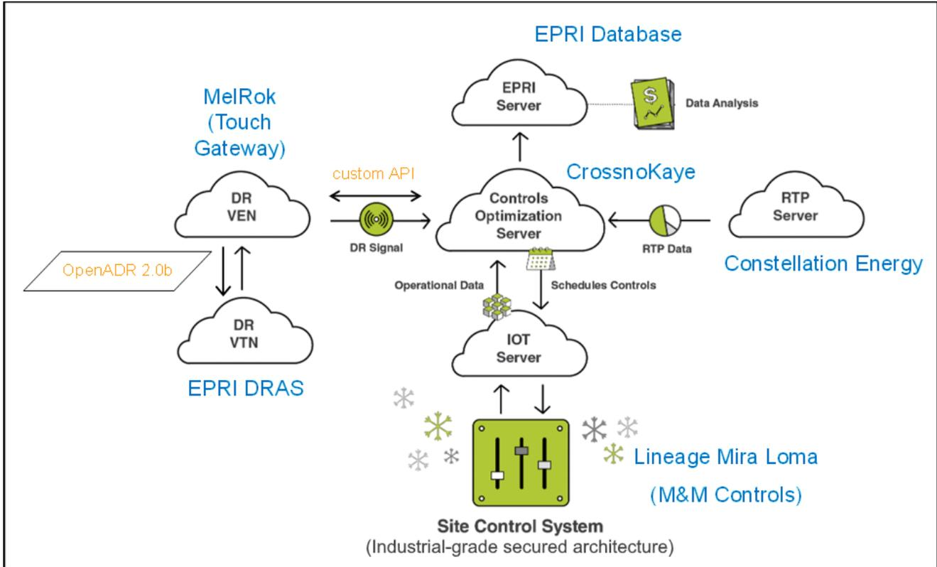
Diagram showing the communication architecture for implementing OpenADR 2.0b on the Lineage refrigeration plant with process optimization
