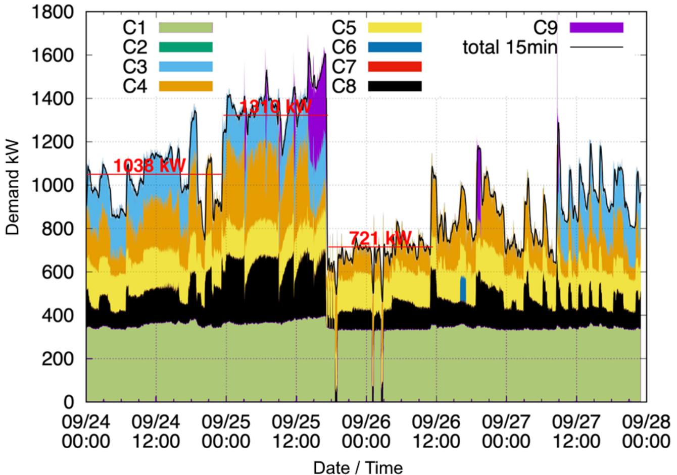
In the improved experimental design, power response of all chillers (C1 to C9) to the DR event consisting of a pre-cool period from 12:00 a.m. to 5:00 p.m. on September 25, 2021, followed by a power-down event until 12:00 p.m. on September 26, 2021 (compressor C7 is inactive)
