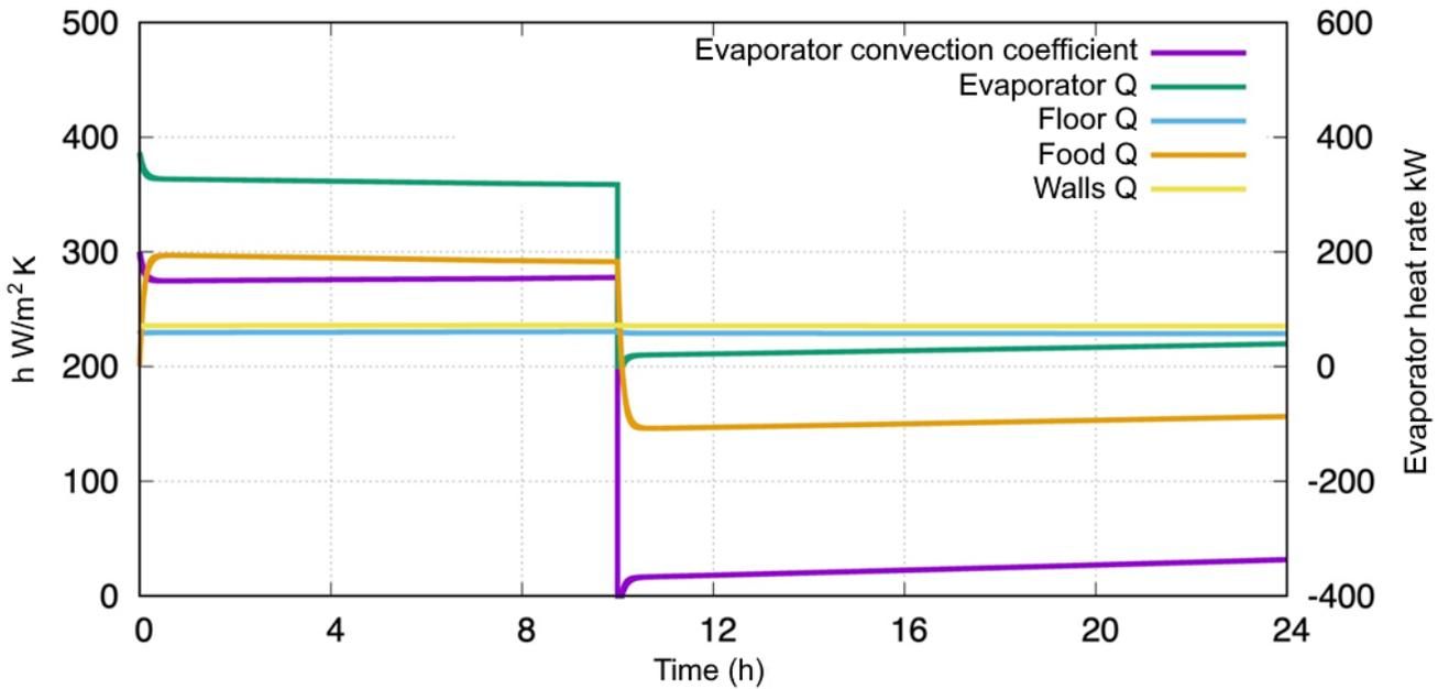
Graph showing the model of a heat transfer process between frozen room components during a DR temperature setpoint reset.
