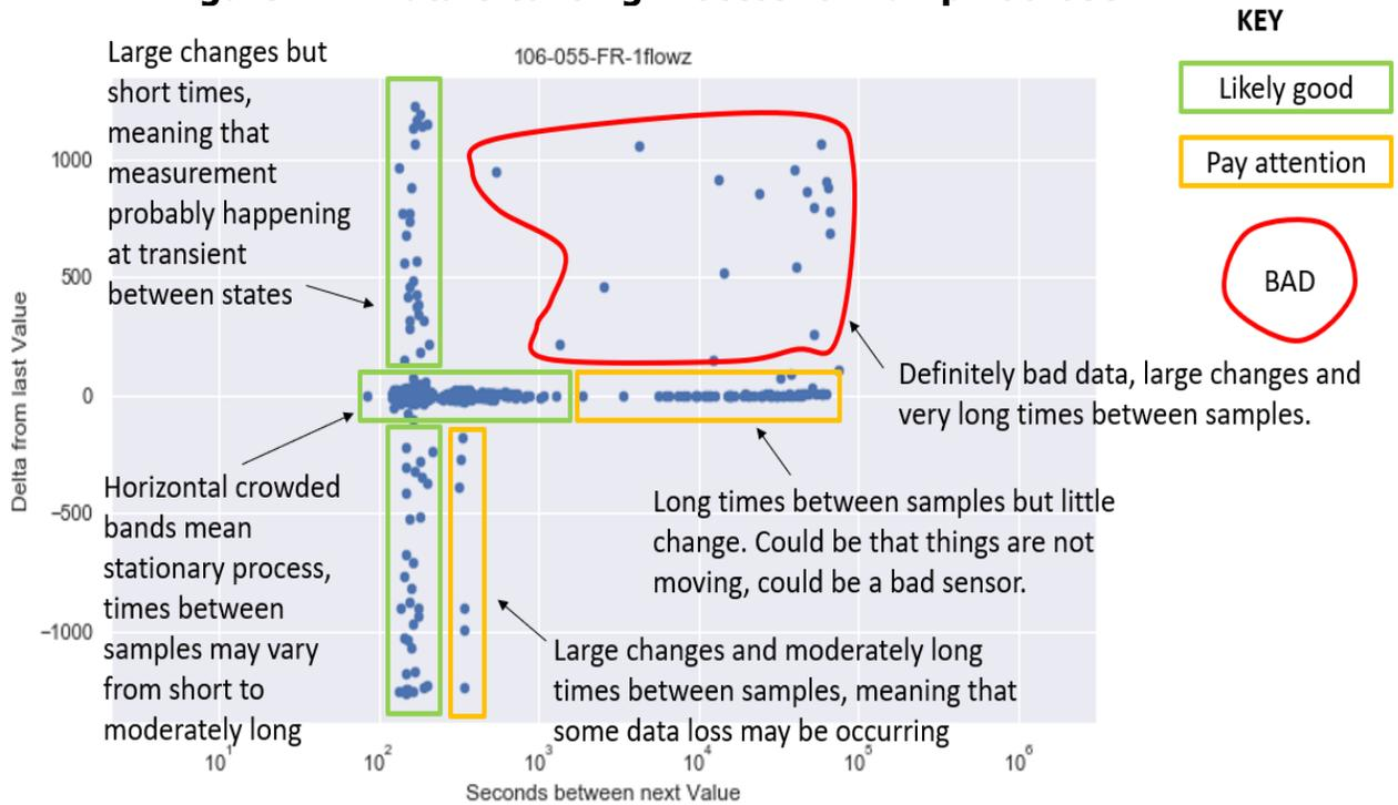
**Graph showing data cleansing process for pump 106-055-FR-1.**
