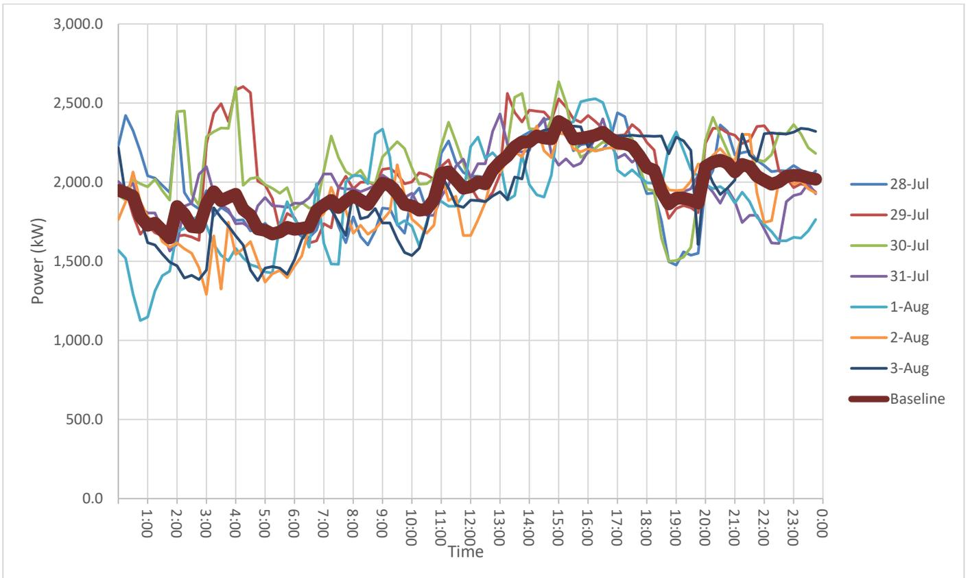
Baseline development for the floor heater DR experiment using entire-site meter data.
