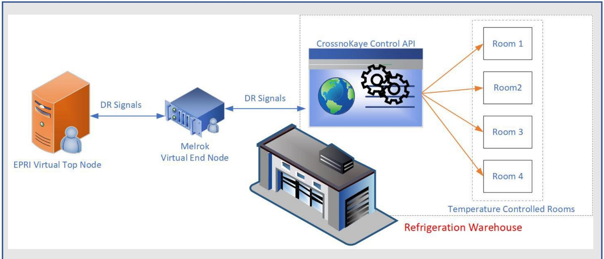
**Diagram of implementing OpenADR 2.0b on the Lineage refrigeration plant with process optimization**
