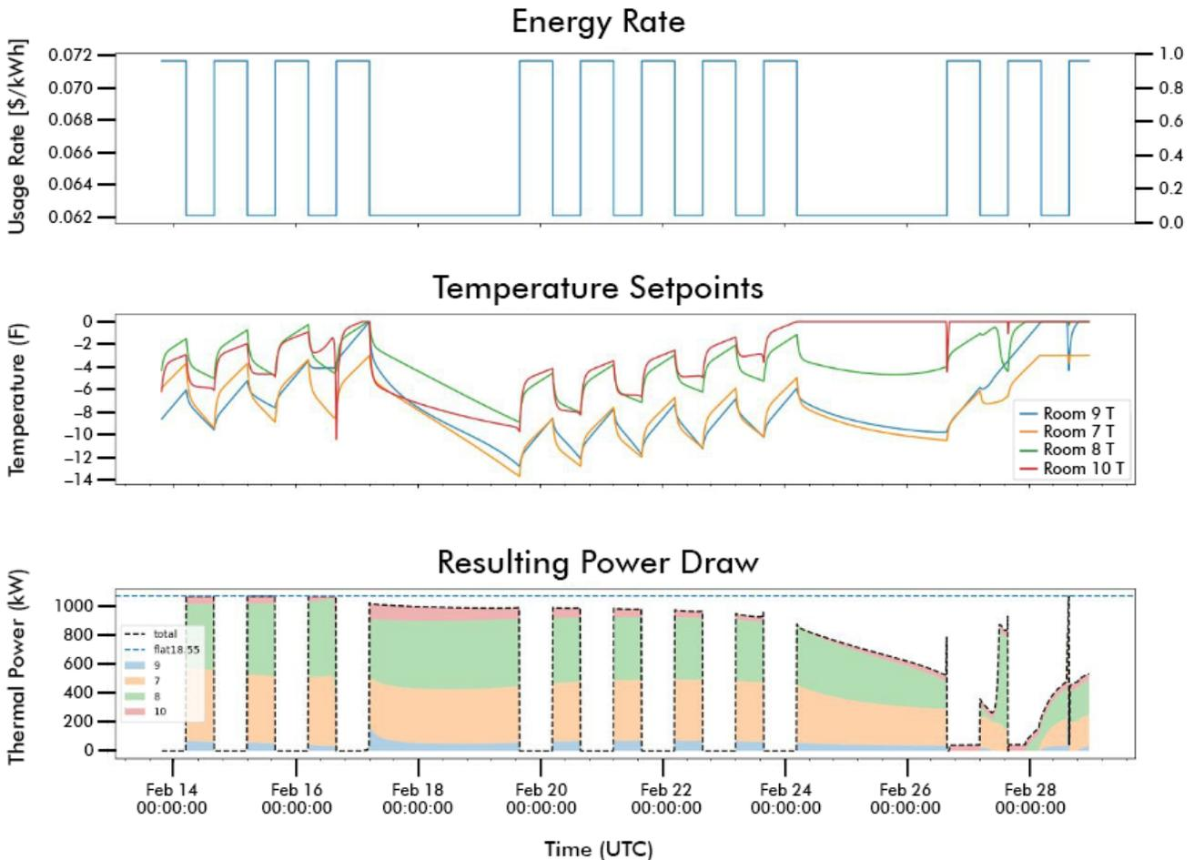
**The diagram shows example optimization and operations schedule for the Lineage refrigeration plant, using the energy price as an input to the optimization process. Note that temperature setpoints are controlled to eliminate energy use during peak energy prices.**
