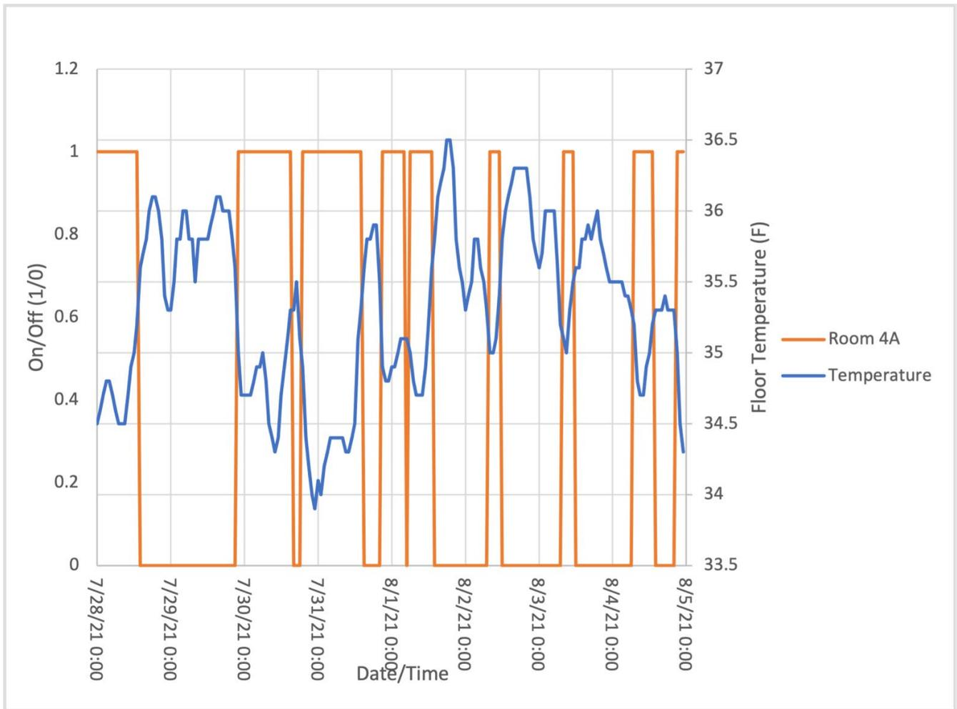
**Graph showing how floor heaters in Room 4A turn on or off according to monitored floor temperature.**
