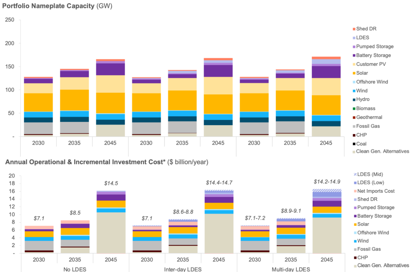
Figure 26: Total Resource Portfolios (top) and System Costs (bottom) Under 0 MMT Policy with Emerging Low-Carbon Generation Alternatives
