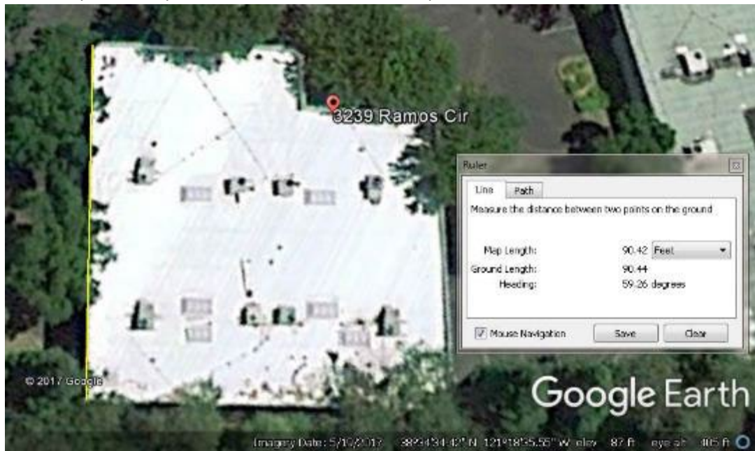
Figure 18. Google Earth™ Satellite View of a Building and a Measurement of One Side.
