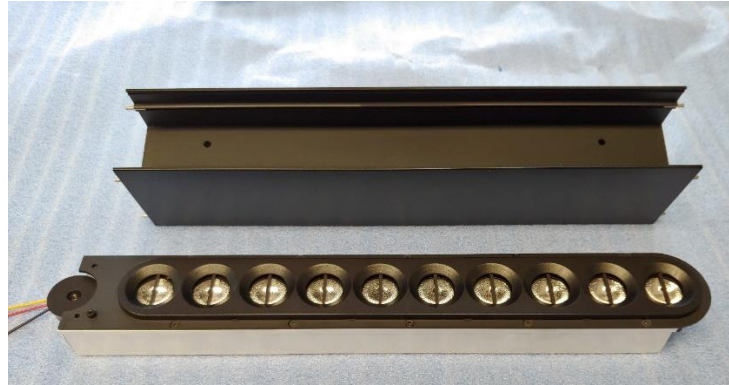
Figure 10: Fully Assembled Core (bottom) Ready for Insertion into Shell (top)
