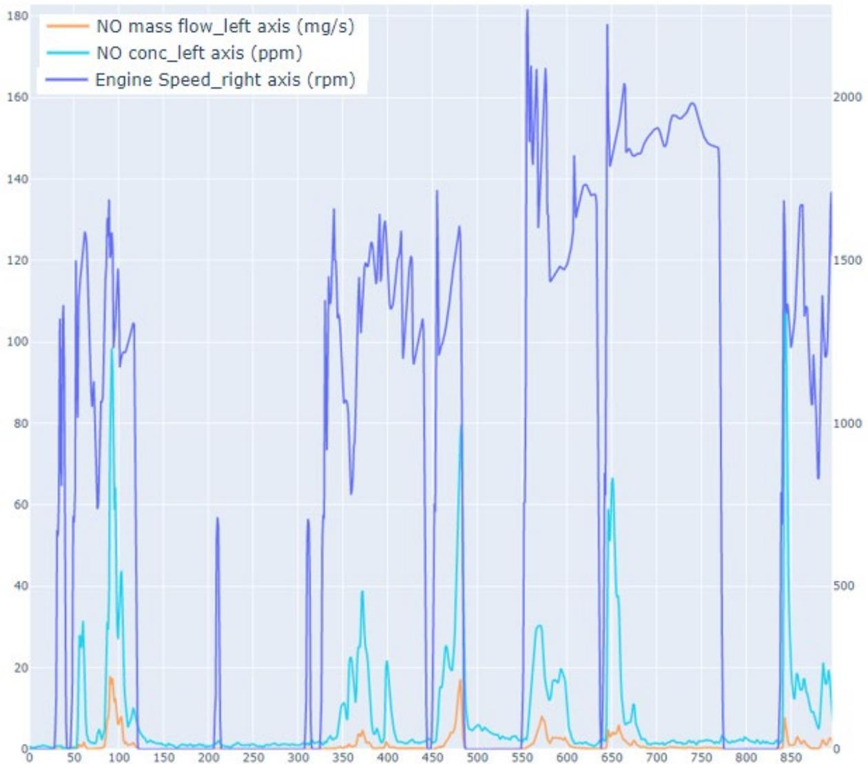
Engine OEM support is needed to understand this behavior and to find a way to control the NOx in the start phase. Once a control strategy for NOx emissions during startup is established, it could be implemented in the model and the start-stop logic may be activated with a simple calibration change in future development which, depending on the operating conditions, may offer up to a 10 percent fuel economy improvement.
