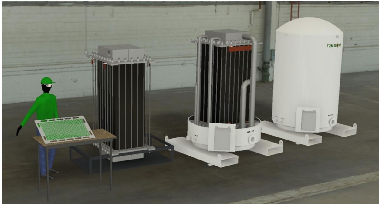
Figure 28. AES Cell to 315 kg/day Stack in Multi-purpose Enclosure
