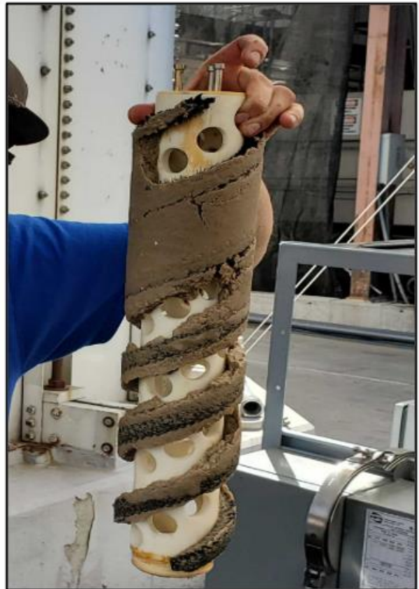
Figure 19: Fouling on Prefiltration System #1 (Left) and on Prefiltration System #2 (Right)
