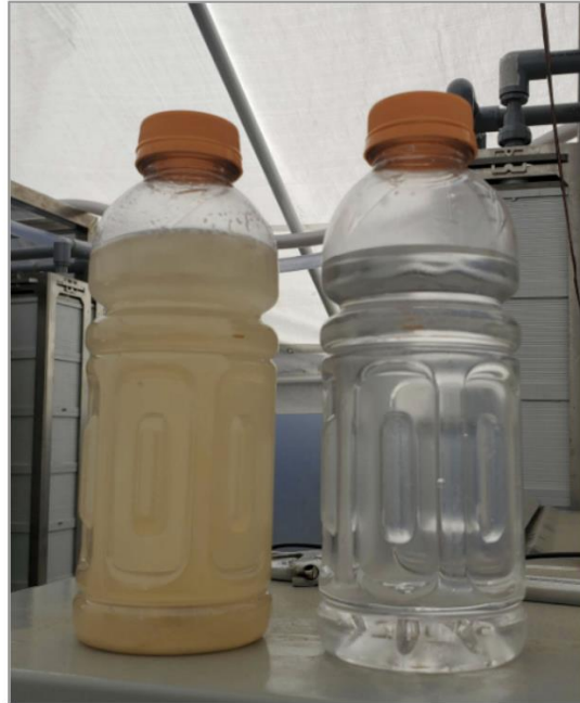
Figure 12: Raw Wastewater (left) and PFO Recycler Permeate (Right)
