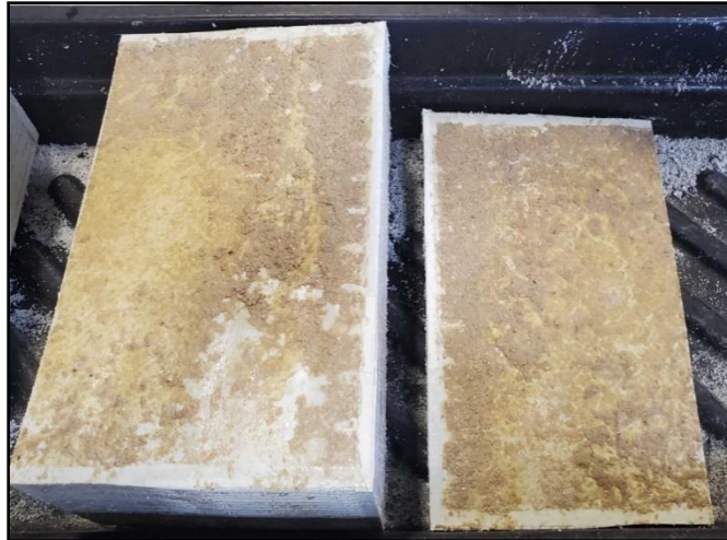
Cut element showing fouling (accumulation of starch solids)
