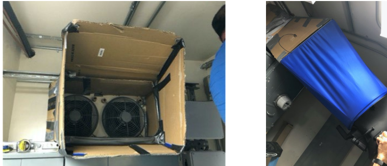
Figure 93: Hood to Convey Air Flow to Flow Measurement Device (Left), and TSI Volumetric Flow Measurement Device in Use (Right)
