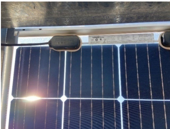
Figure 16: Bifacial Module Back Sheet
