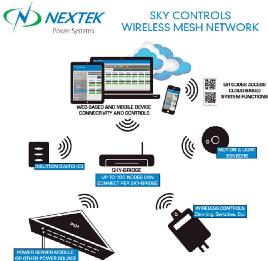
Figure 102: Lighting System Components
