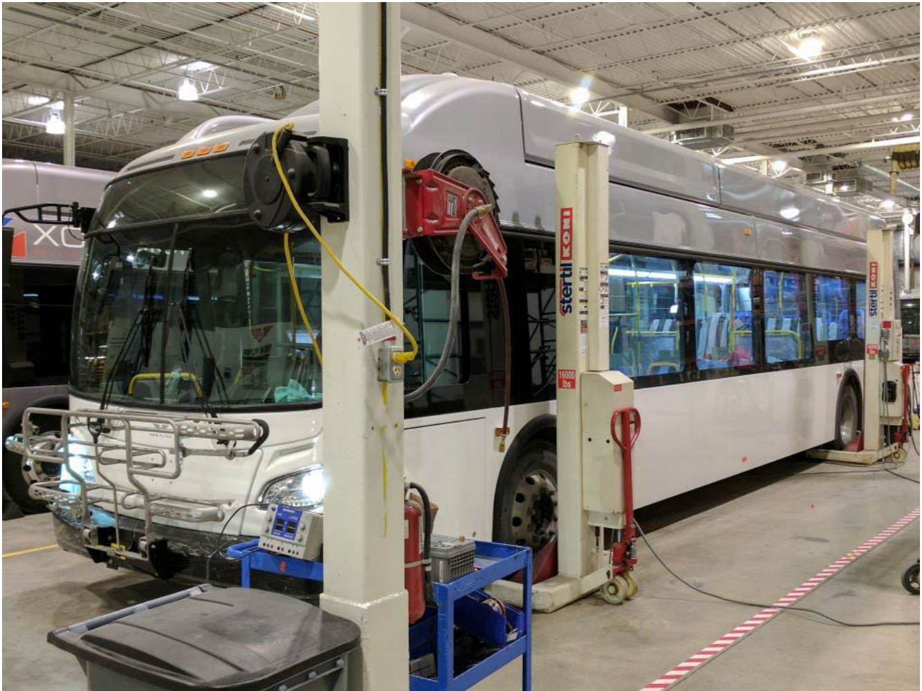
Figure 31: Completed Hydrogenics Advanced Fuel Cell Bus
