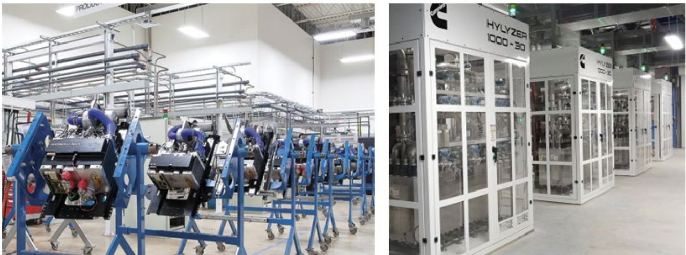
Figure 1: Hydrogenics' Fuel Cell Manufacturing Line (left) and Electrolyzer Installation in Bécancour, Canada (right)
