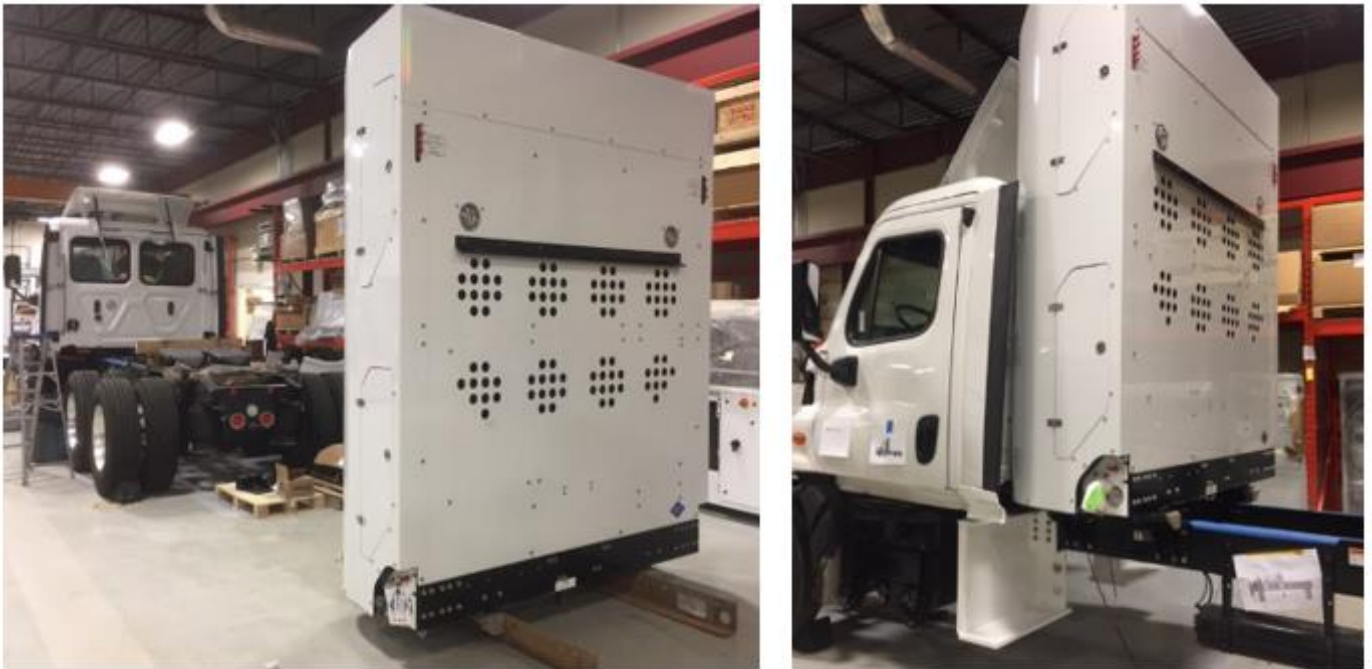
Figure 30: Hydrogen Tank System Installation
