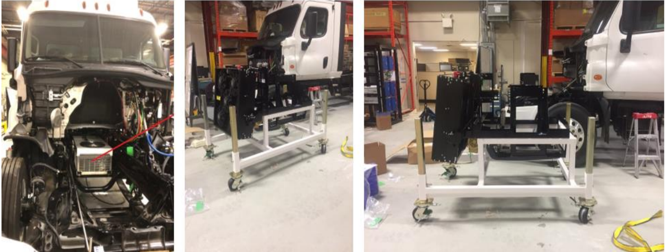
Figure 28: Battery Chiller Installation (left) and Fuel Cell Cradle Preparation (right)
