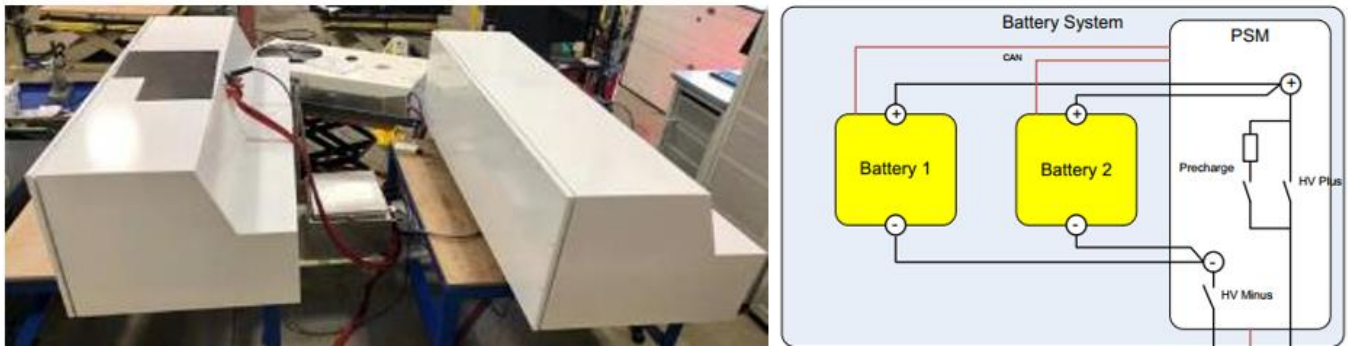
Figure 15: ACTIA High Volt Battery Enclosures (left) and System Architecture (right)
