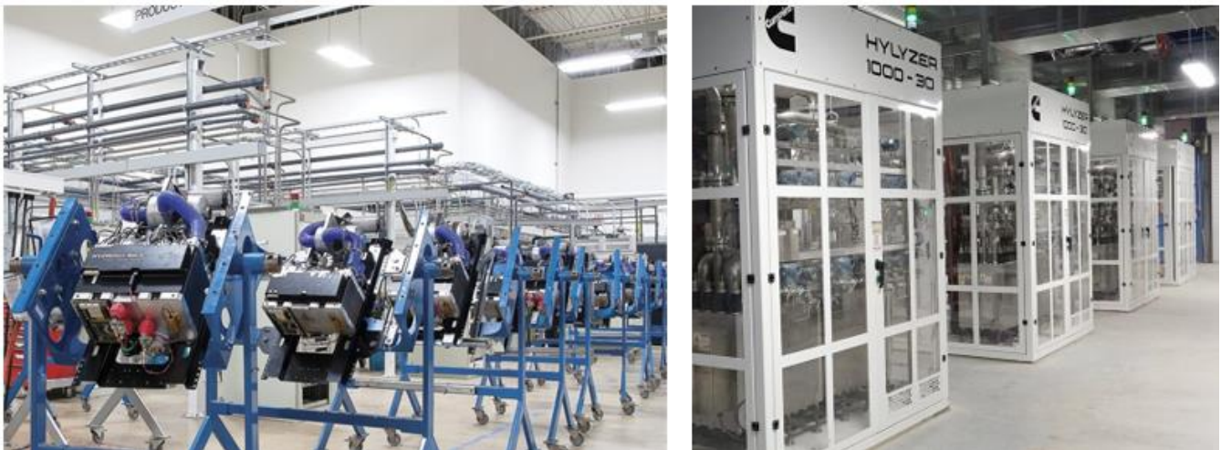
Figure 1: Hydrogenics' Fuel Cell Manufacturing Line (Left) And Electrolyser Installation in Bécancour, Canada (Right)
