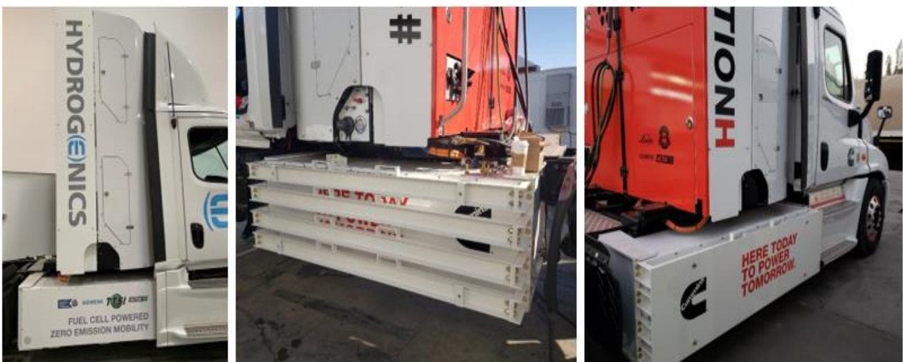
Figure 39: Original High Voltage Battery Pack Design (left) and with Crash Protection Bracket (middle and right)
