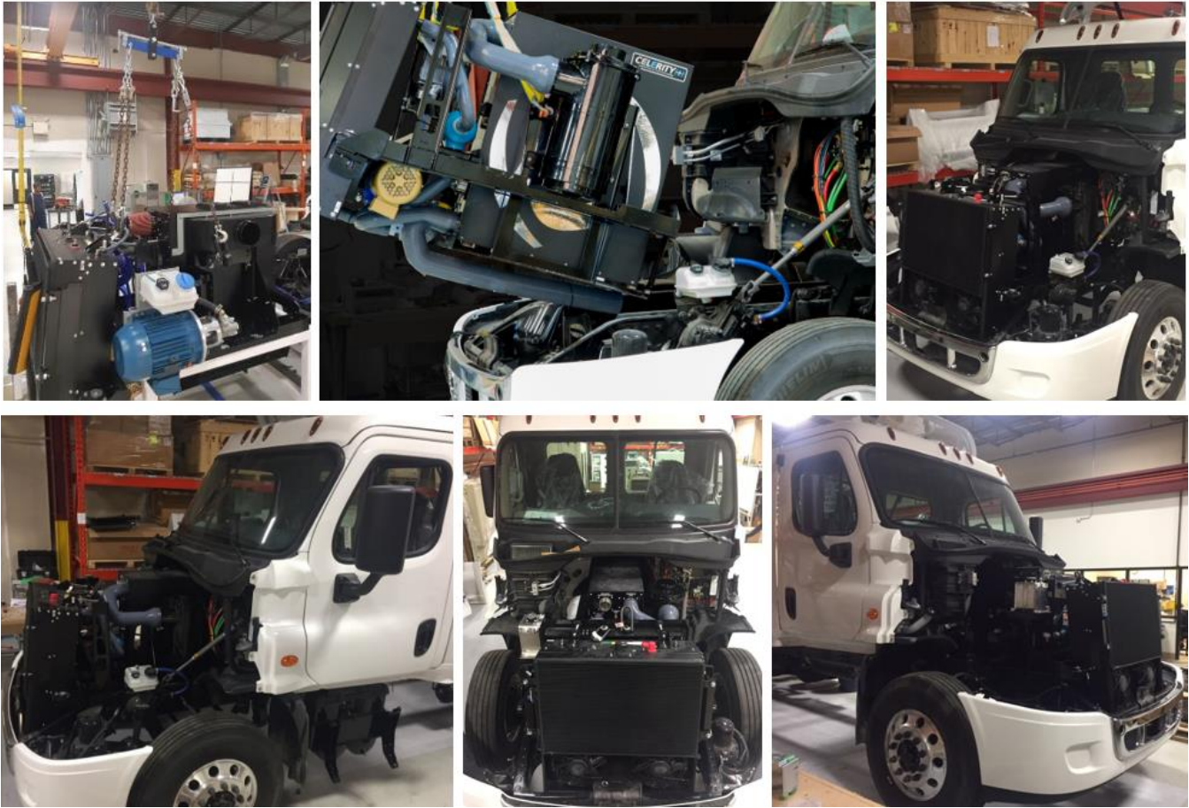
Figure 29: Hydrogenics Celerity Plus Subassembly Installation
