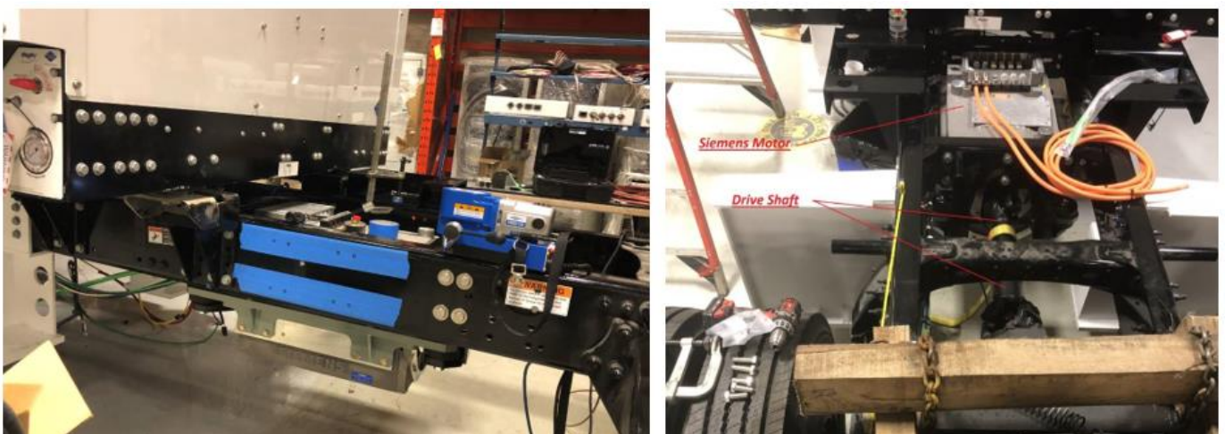
Figure 31: Drive Motor and Drive Shaft Installation
