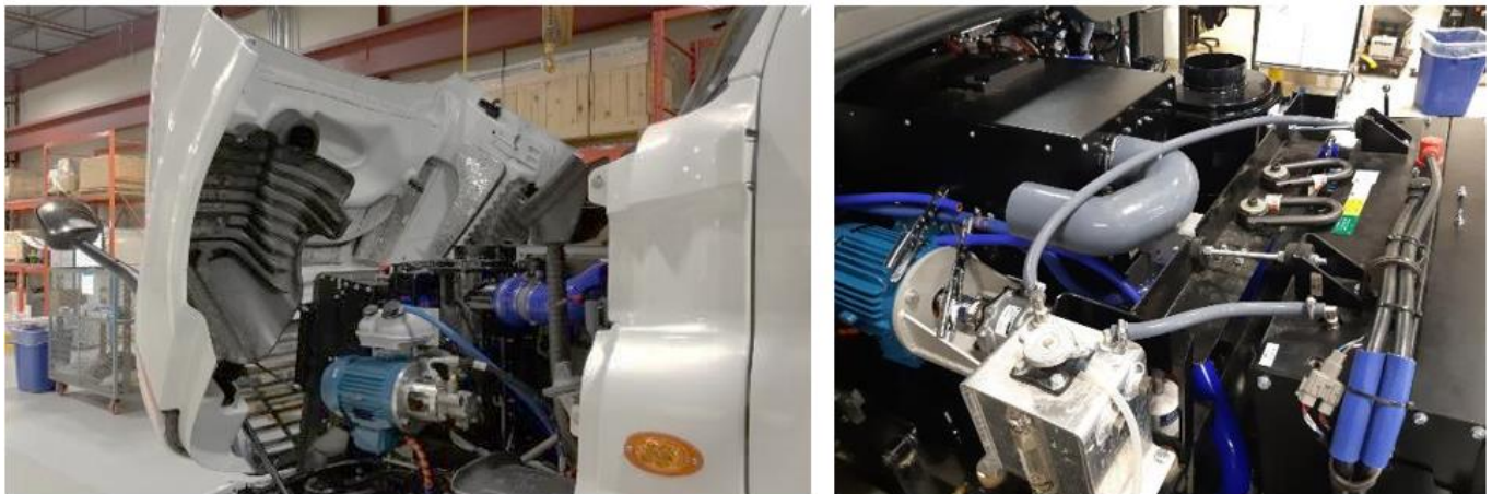
Figure 9: Hydrogenics Celerity Plus Subassembly Installed in Truck Engine Bay
