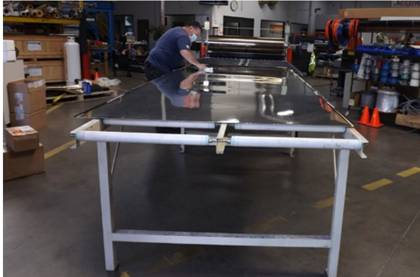
Figure 21: Mirror panel lamination
