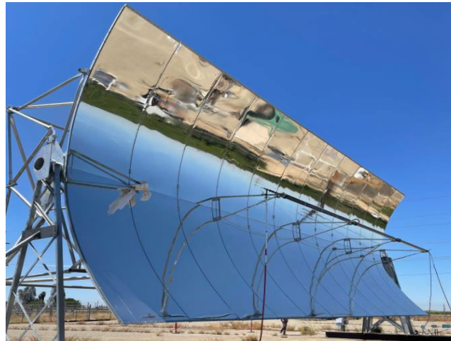
Figure 31: Three, 4-meter-long receivers with new secondary reflectors mounted for on-sun optical efficiency testing
