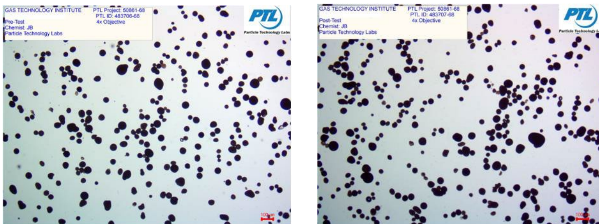
Figure 53: Four times micrographs of pre-(left) and post-test particle samples
