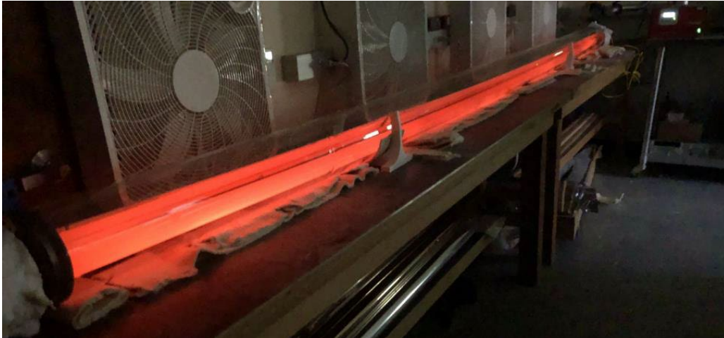
Figure 17: Receiver undergoing 100-hour testing at 1,202 °F (650 °C)
