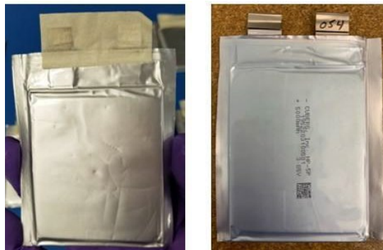
Figure 2: Cell That Failed Quality Control (left) and Cell That Passed (right)
