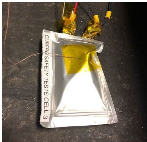
Figure 7: Cuberg Cell Following 8-hour Overcharge at 1.5A
