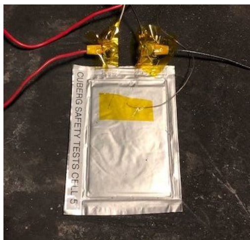
Figure 6: Fully Charged Cell After External Short Circuit Test at Room Temperature
