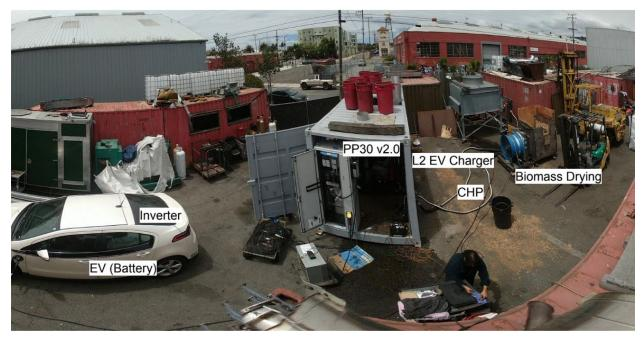
Figure 25: Layout of MG1002 During EVT Testing at APL Berkeley
