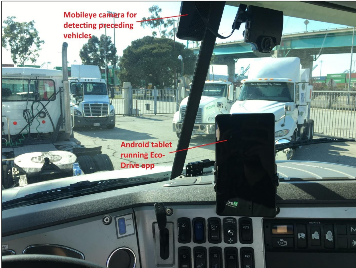
Photo showing the Eco-Drive System installed on a truck of the participating fleet
