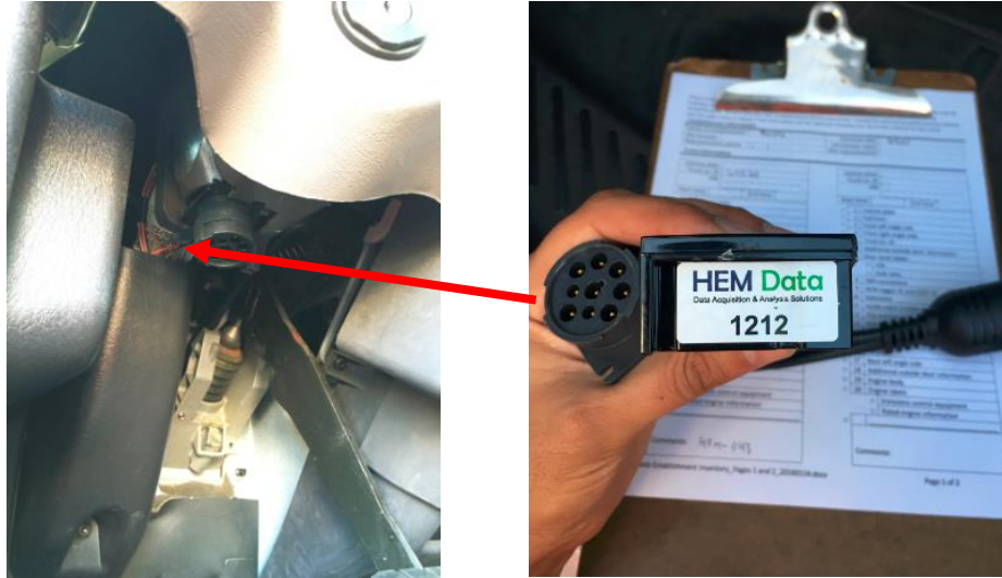
Photos showing the J1939 Mini Logger™ used for data collection and ECU port on a truck Credit: University of California, Riverside
