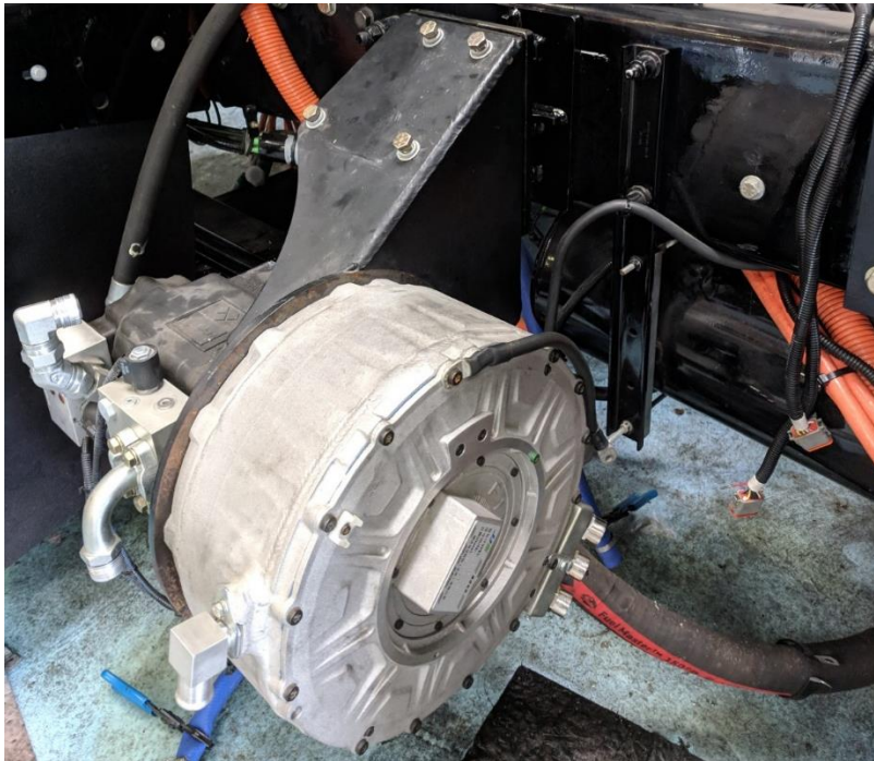
Figure 4: ePTO Installed on the Glider Chassis
