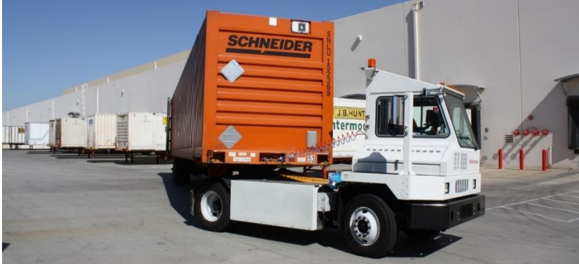
Figure 6: Battery-electric Kalmar Yard Tractor with 400Ah CALB ESS
