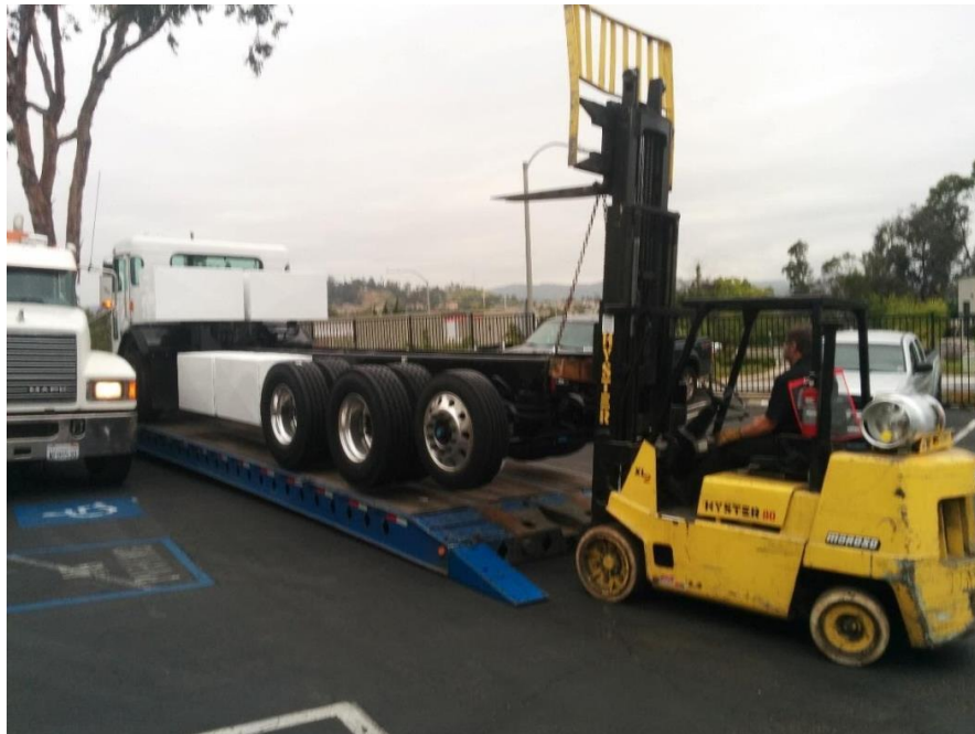
Figure 18: Truck Chassis Being Loaded on a Flatbed to Ship to Body Installer
