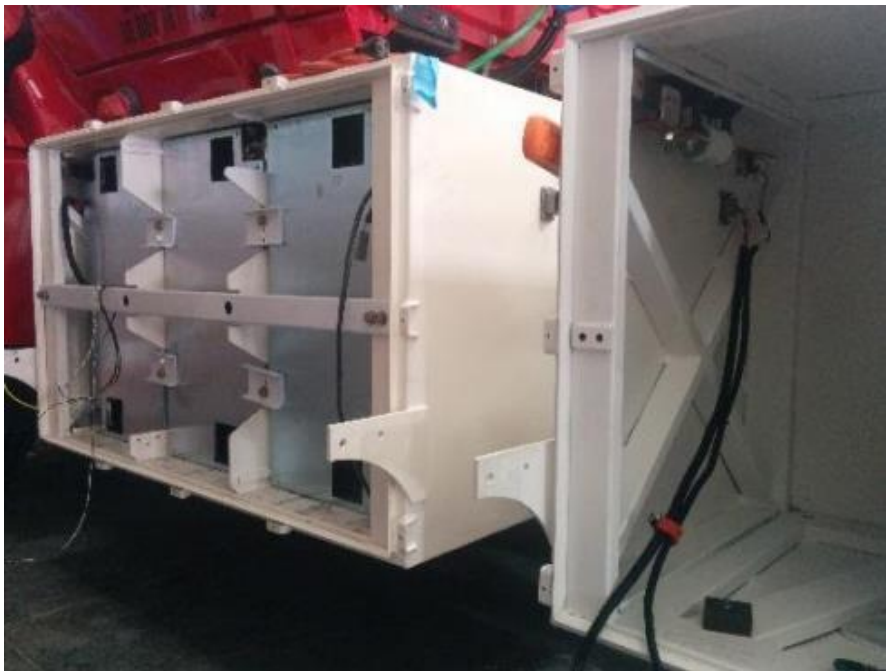
Figure 11: KAM Modules Mounted in Enclosures on a Test Vehicle
