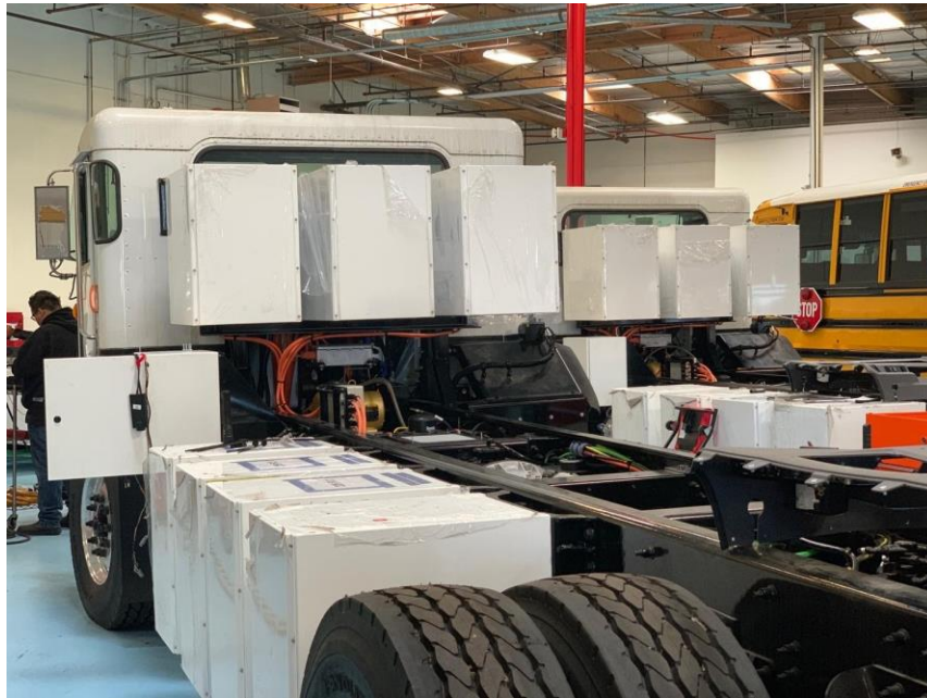
Figure 15: Peterbilt 520 with Seven Strings of the NMC ESS
