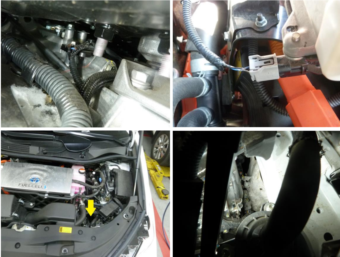
Figure 24: Rodent damage to the wire harness on four Mirai Vehicles
