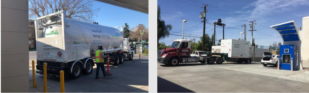
Figure 1: Liquid Hydrogen and Gaseous Hydrogen Delivery Trucks
