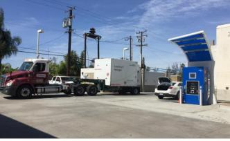
Liquid hydrogen truck can deliver 2,400 kg (left) compared to 120 kg for gaseous hydrogen truck (right). Source: FirstElement Fuel, Inc.
