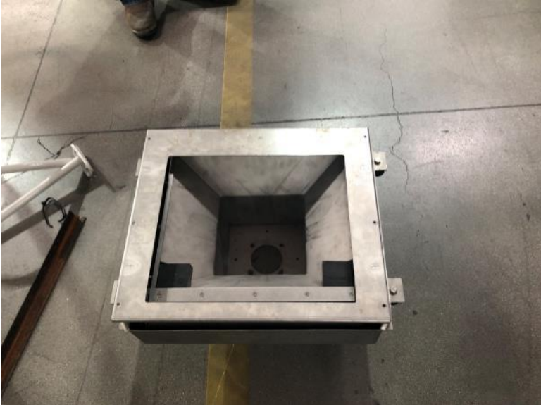
Figure 4 - Cavotec SPS Plug Module Funnel for the BYD 8Y Yard Tractor
