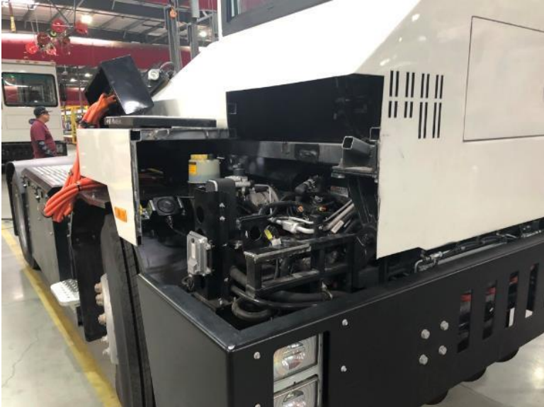
Figure 3 - Cavotec SPS Plug Module Integration into BYD Electric Yard Tractor
