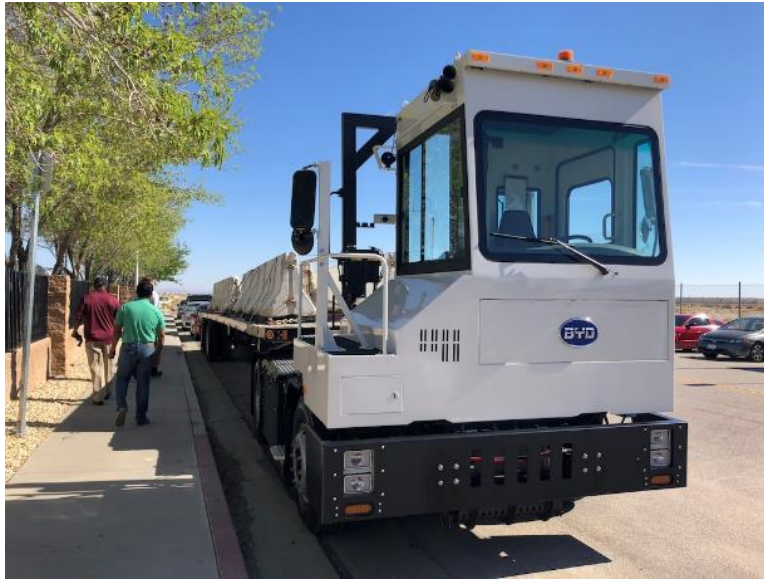
Figure 12 - BYD Electric Yard Tractor Validation Testing at BYD Lancaster Facility
