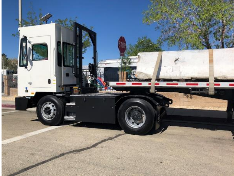
Figure 14 - BYD Model 8Y Undergoing Acceleration Validation Testing
