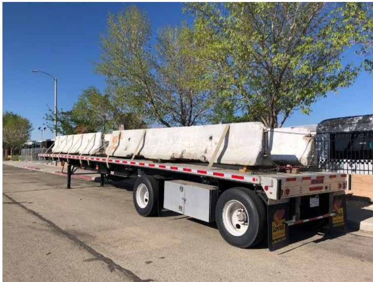
Figure 13 - Simulated 70K GCW Container Used in Pre-Deployment Validation Testing
