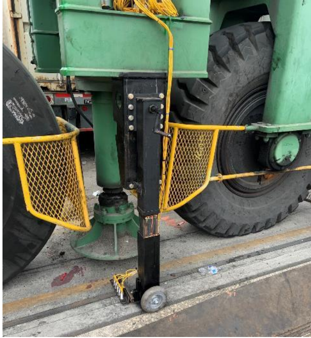
Figure 9 - eRTG Mounted Arm with Proximity Switches
