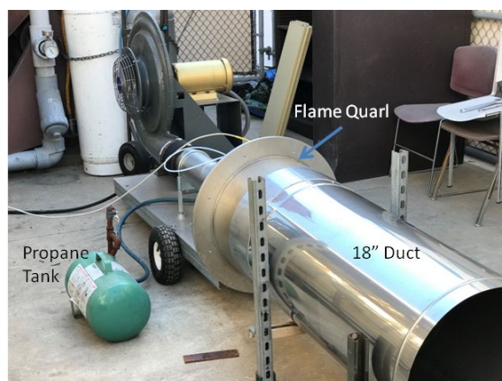
Figure 46: Setup to Commission Full-Scale LSB Using an 18" Steel Duct to Simulate Combustor Enclosure
