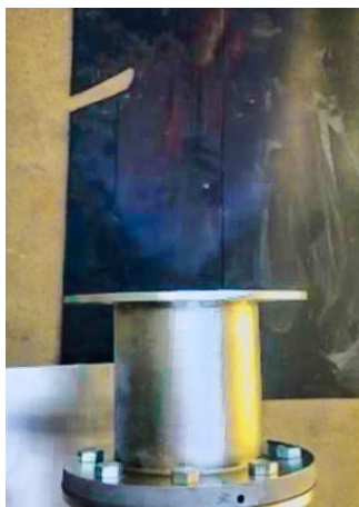
Figure 45: Lean Methane/Air Flame Generated by the Full-Scale LSB Prototype
