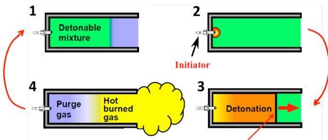
**Figure 6: Pulse Detonations at 20-Hz**
