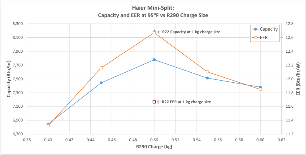
Figure B-3: R-290 Charge Optimization Test Results for the Haier Mini-Split Air Conditioner
