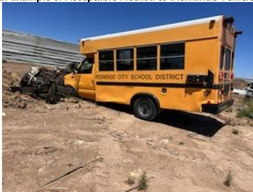
Figure 2: Example of Acceptable Method to Dismantle Vehicle Chassis
