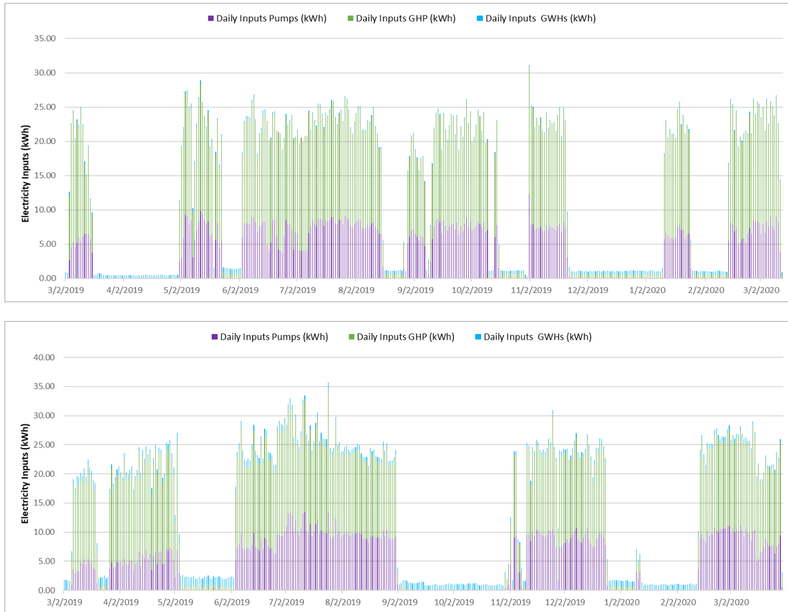
Figure D-17: Electricity Input to Gas Heat Pump System Components at Site #1 (Top) and Site #2 (Bottom)
