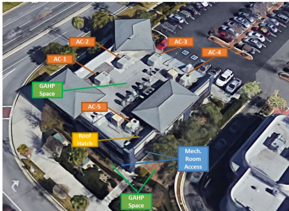
Figure C-20: Location of Heating, Ventilation, and Air-Conditioning Equipment on Rooftop and Potential Gas Heat Pump Locations
