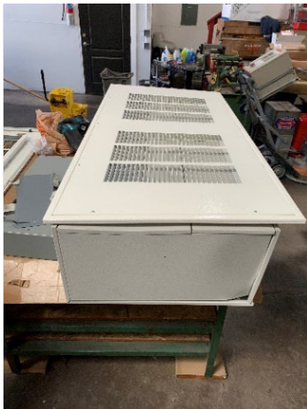
Figure D-9: Damaged Fan Coil Unit Upon Receipt (Left) and Targeted Restrictions at Site #2 (Right)
