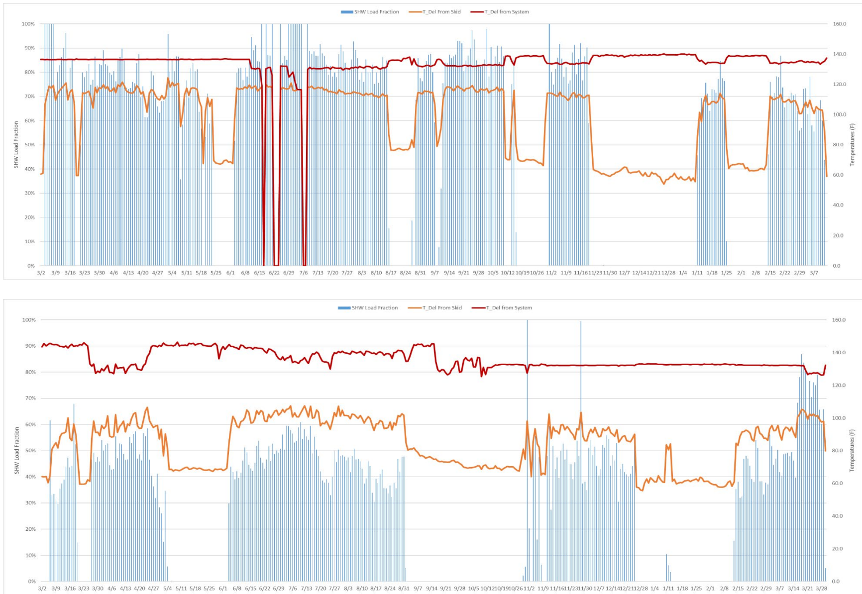
Figure D-15: Service Hot Water Load Fraction for Gas Heat Pump, with Delivered Temperature from Skid (to Gas Water Heaters) and from System for Site #1 (Top) & Site #2 (Bottom)
