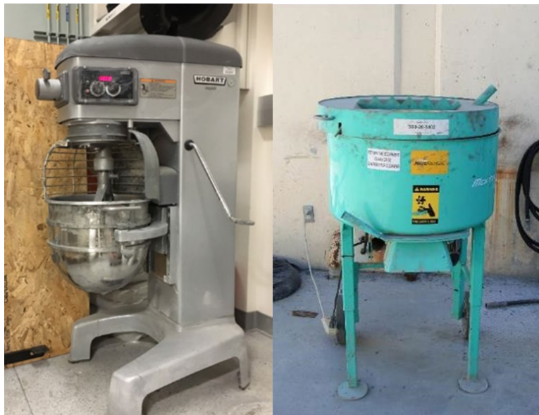
Figure 17: Concrete Mixers With Different Capacities for 3DCP
