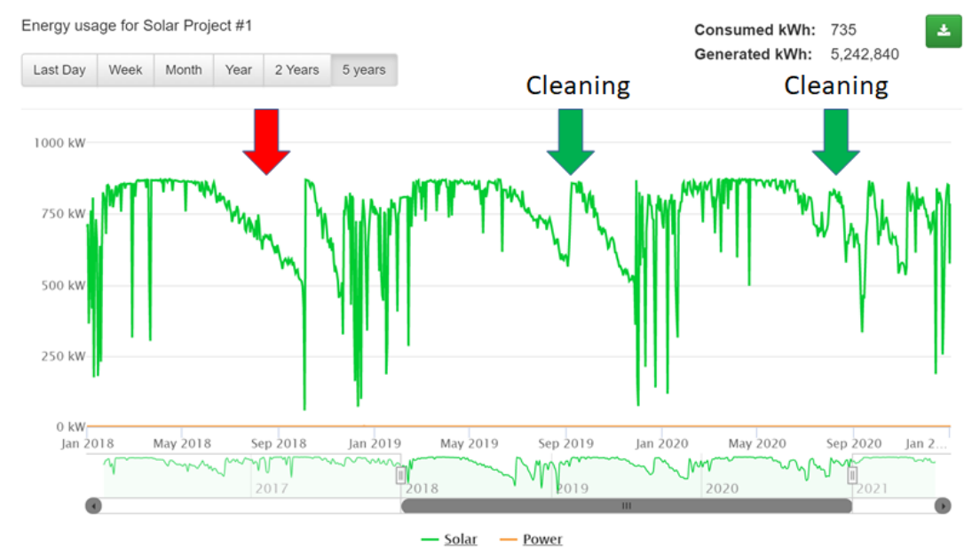
Figure 58: Production of Solar Energy at Farm #12 With and Without Cleaning
