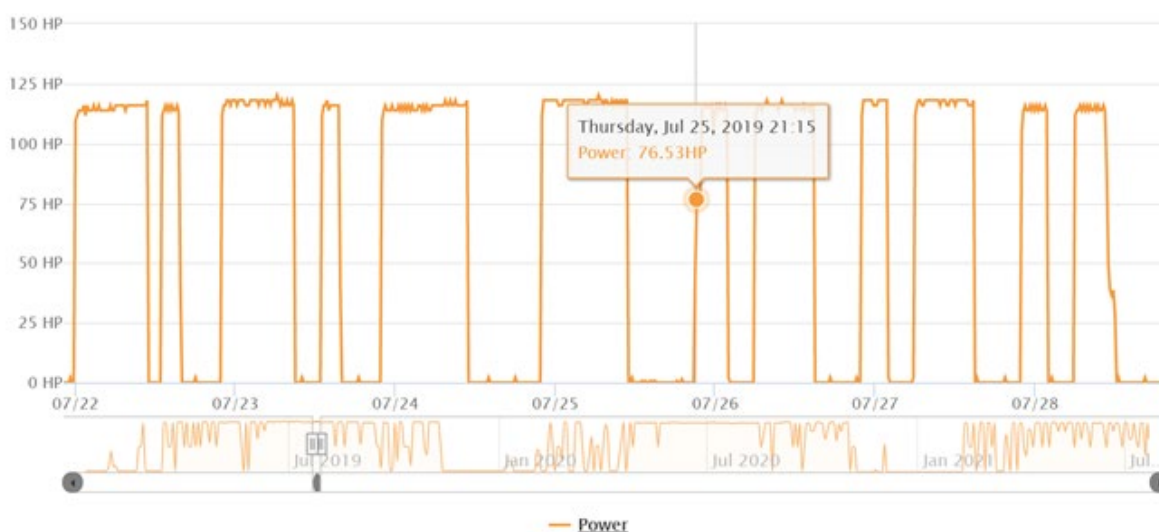
Figure 55: Interval Data from SmartMeter for a Pump Station Used to Irrigate Outside Peak Hours
