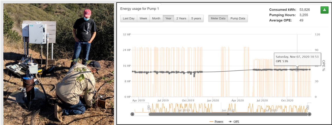
Figure 80: SCE Pump Tester at Farms Near Ventura and SmartMeter Data Showing Improved Pump Efficiency After a Pump Retrofit
