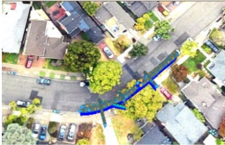
Figure 27: Projections of Surface Footprints of BakhtarRadar Traces and GPS Coordinates on Google Map
