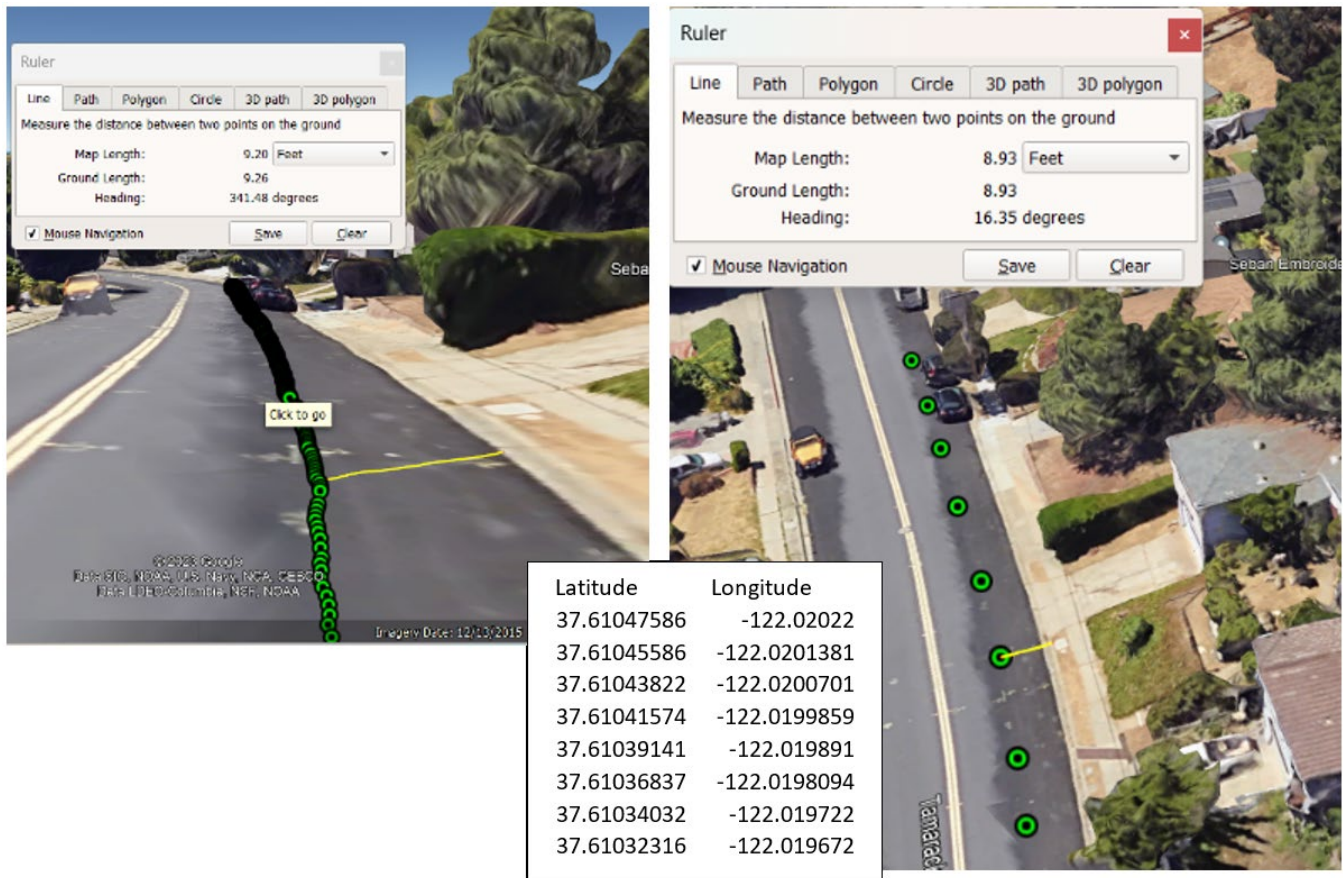
Figure 51: Distance from Curbs to Surface Footprints of Buried Plastic Pipeline Averaging 9.0 Feet Tamarack Drive Union City
