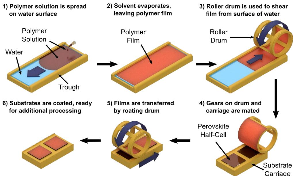
**A polymer film is formed on the surface of water before being sheared from the water surface using a cylindrical drum. The freestanding film can then be subsequently transferred to a solid substrate.**
