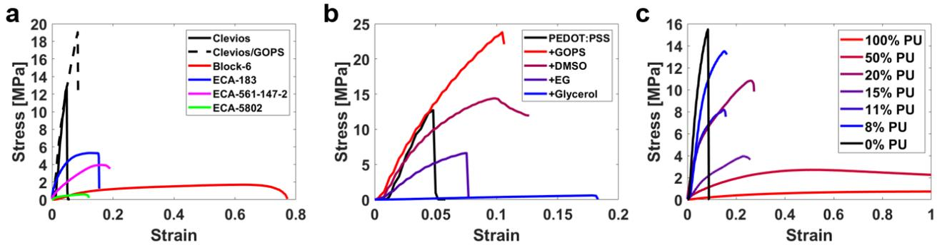
**(a) Different polymer formulations used as conductive adhesives, (b) PEDOT:PSS blended with different secondary dopants (DMSO, EG, glycerol) or crosslinker (GOPS), and (c) PEDOT:PSS blended with different ratios of polyurethane (PU).**
