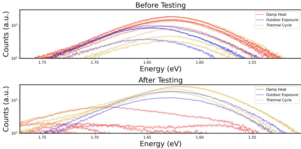
**Before (above) and after (below) degradation testing.**
