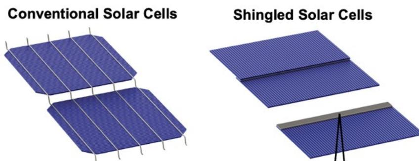
**Traditional module integration (left) uses tabbing wires soldered to busbars to carry current from the back contact of one cell to the front contact of the next cell to wire the cells in series. A shingled module lay-up (right) overlaps the front and back contacts of the cell and connects them with an electrically conductive adhesive.**
