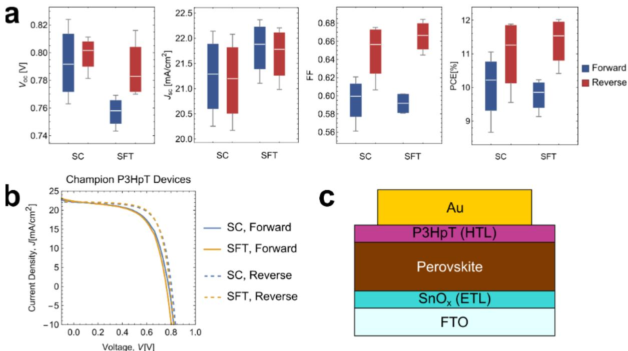
**a) Photovoltaic metrics of perovskite solar cells using a P3HpT hole-transport layer deposited by solvent-free transfer (SFT) or spin coating (SC). b) JV curves of the champion devices made using the two different deposition methods. c) Architecture of the device stack.**
