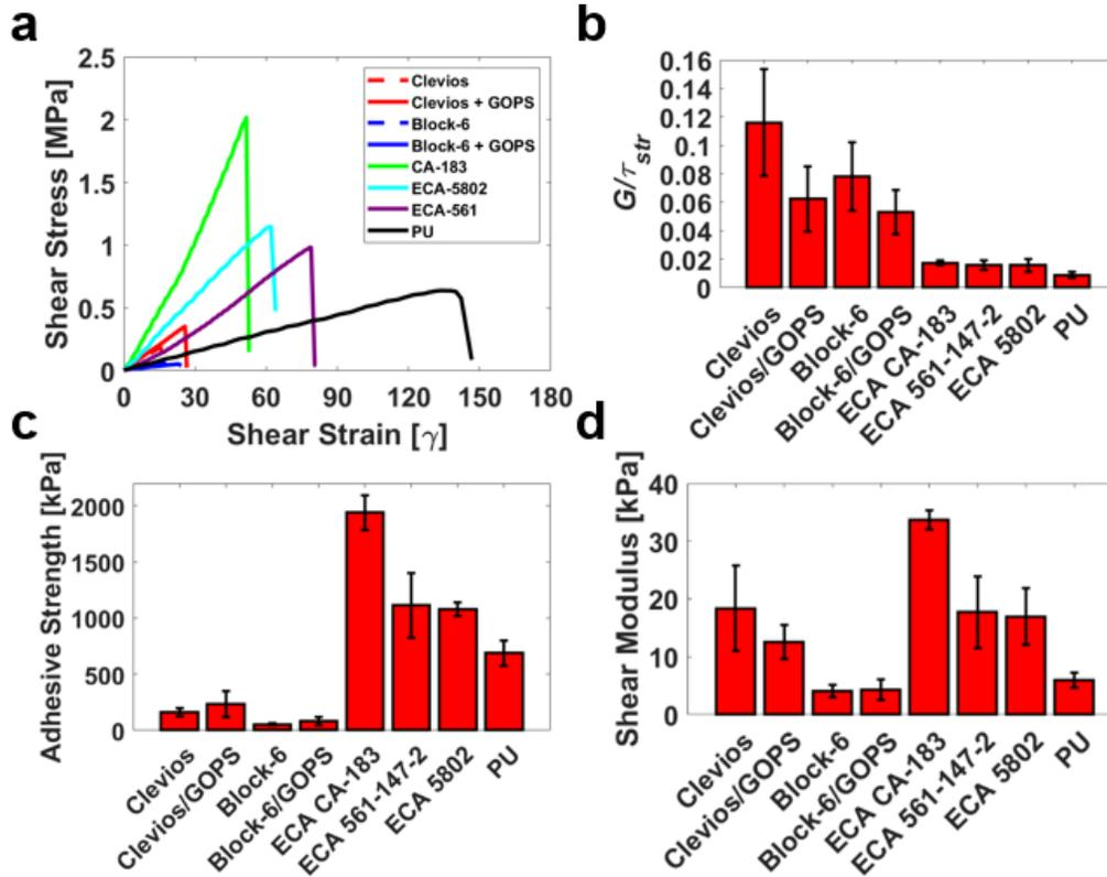
**(a) Representative shear stress-strain measurements for different adhesives tested in this work. (b) Comparison of the ratio of shear modulus and shear strength, which is an important figure of metric for understanding adhesive behavior. This ratio was calculated from the extracted (c) shear strength and (d) shear modulus.**
