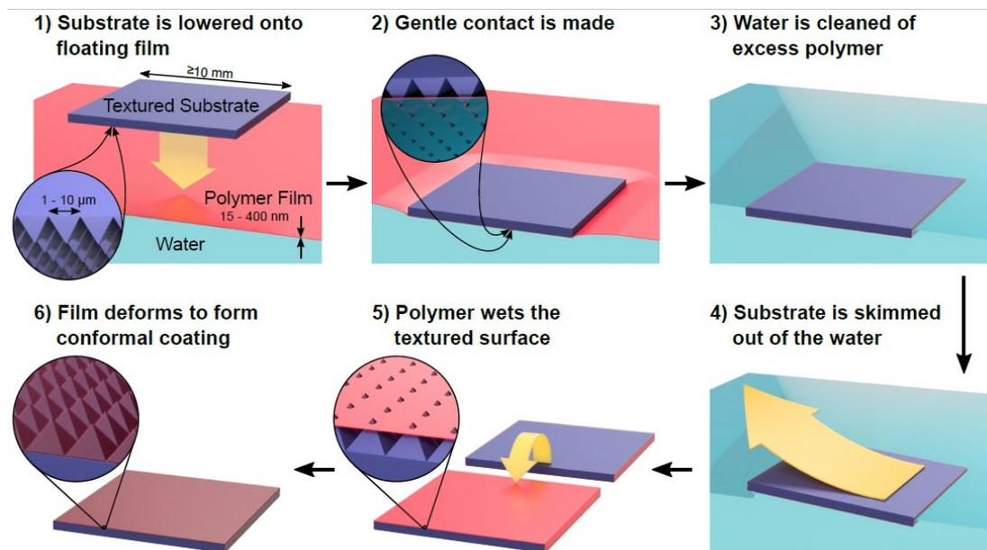
**Taking place in ambient conditions. A polymer film suspended on water is taken up by a textured substrate with high-energy surfaces, enabling the necessary deformation of the polymer as it conformally coats the substrate.**
