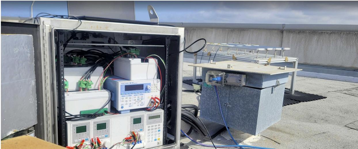
**An electronic weatherproof enclosure (front left) contains measurement equipment with pass-through leads to modules (back right).**
