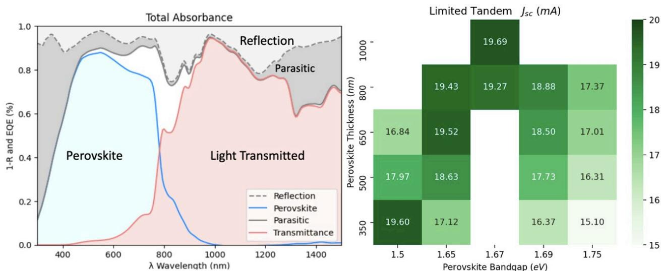
**External Quantum Efficiency (left). The limiting current (right), obtained by conducting a parameter sweep over the absorber bandgap and the thickness of the top cell.**
