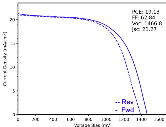
**ITO/Silicon/ITO/MeO-2PACz/Perovskite Absorber/C60/SnOx/ITO/Silver architecture.**
