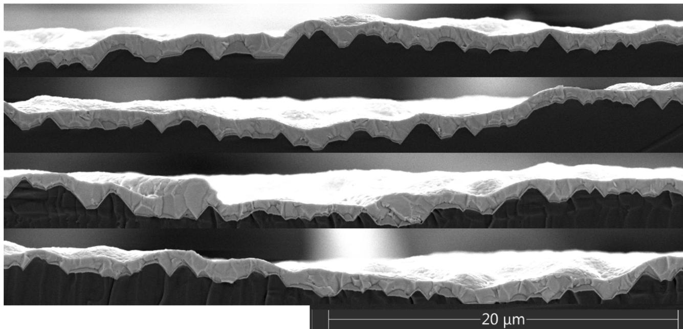
**Perovskite thickness of  $1.0\mu\text{m}\pm 0.3\mu\text{m}$ , scale bar  $20\mu\text{m}$ .**
