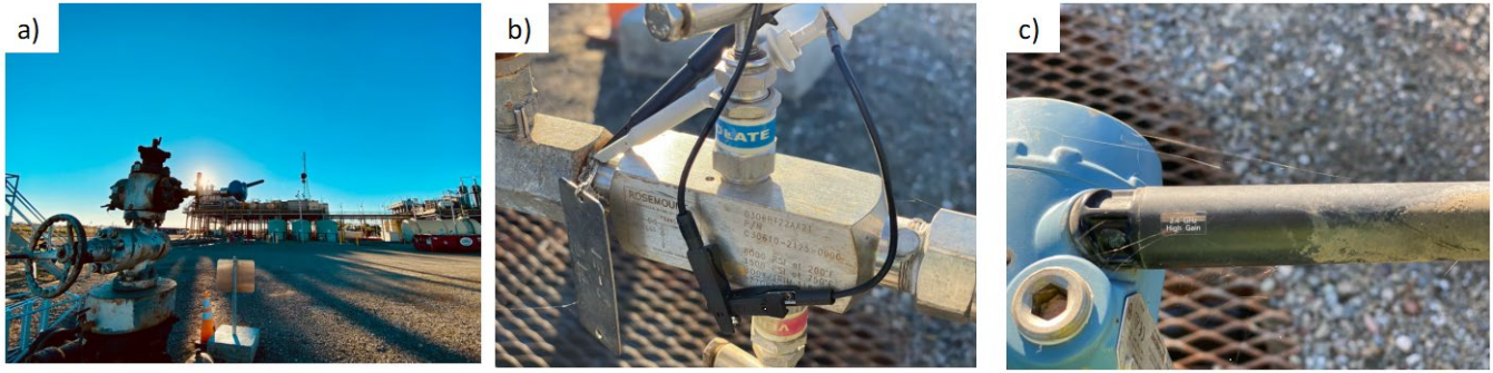
(a) The wellhead of the tested wellbore. (b) The pressure valve on the wellhead was used for sending and receiving electromagnetic waves. (c) The communication antenna on the wellhead.
