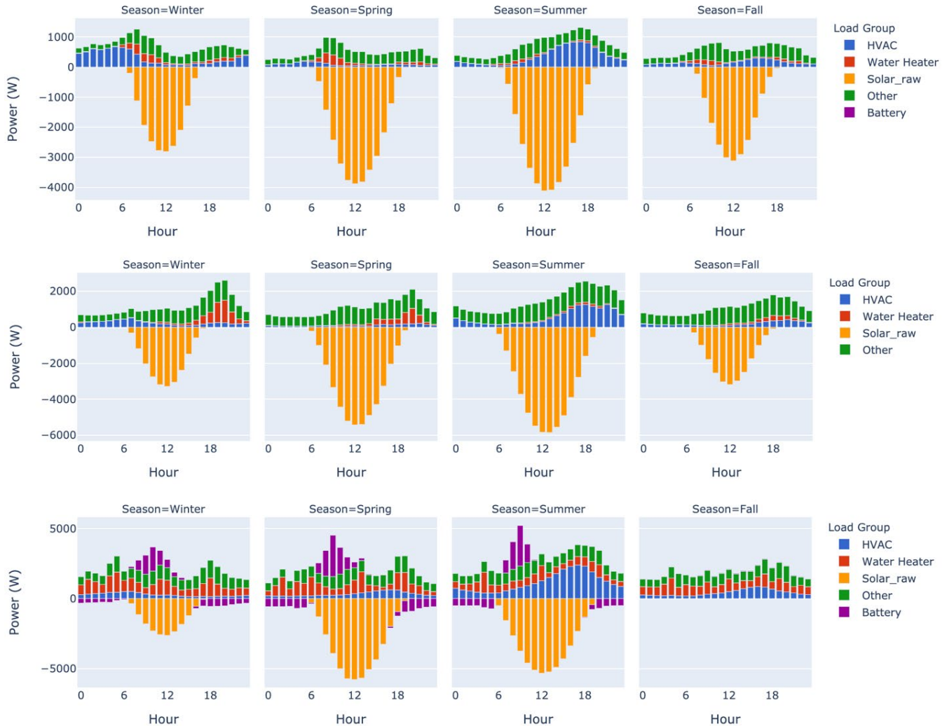
Figure 21: Home-Level Load Shapes Split by Load Group From Three Clovis Homes in 2020
