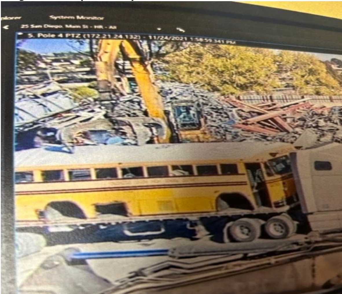
Figure 2: Example of Acceptable Method to Dismantle Vehicle Chassis
